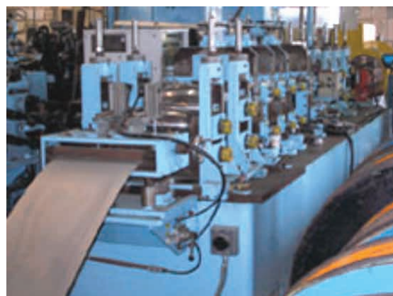
Figure 2 Automatic continuous manufacturing machine for thin-wall metal pipes.
