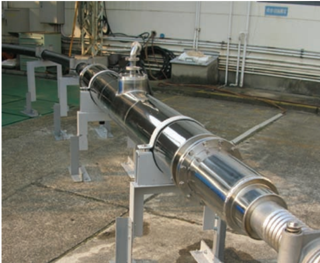
Figure 9 Normal joint for superconducting power cable.
