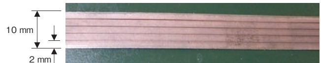
Figure 4 YBCO tape divided into 2 mm in width.
