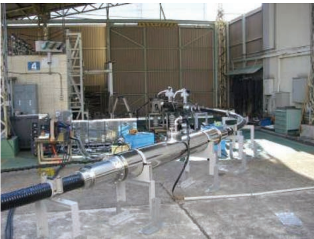
Figure 13 Fault current test of 20-m long superconducting power cable.
