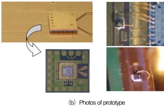
**Figure 3 Simple mounting structure of optical module on OE-PWB.**
