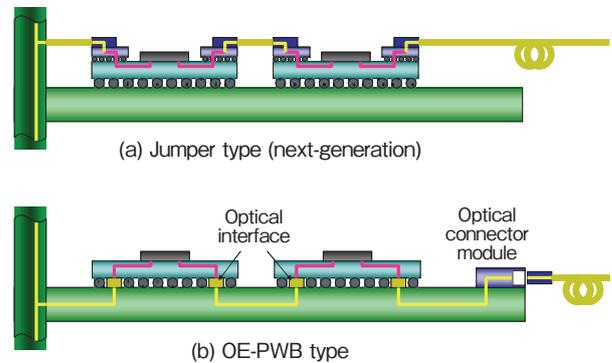
Figure 2 Schematic view of interconnection (II)
