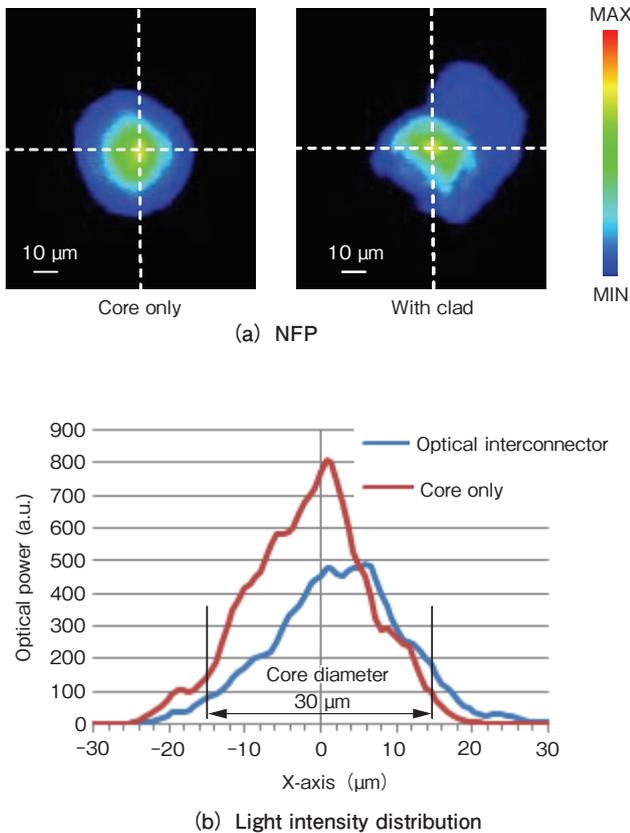
Figure 8 NFP and light intensity distribution.
