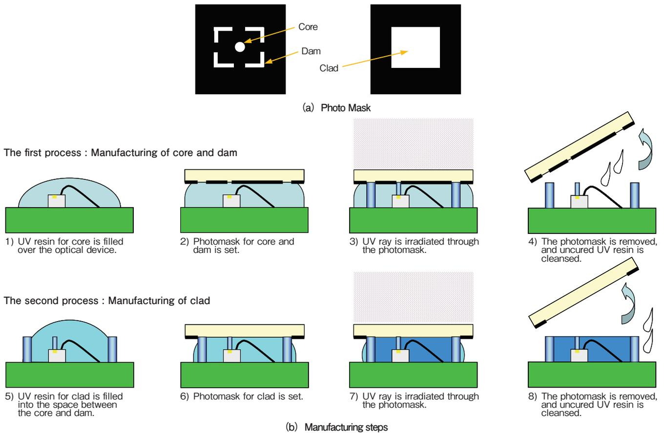
Figure 5 Manufacturing method of optical interconnector.
