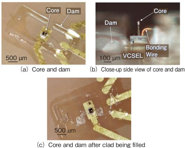
Figure 6 External views of prototyped optical interconnector.
