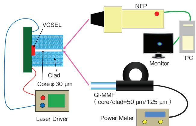
Figure 7 Measuring system.
