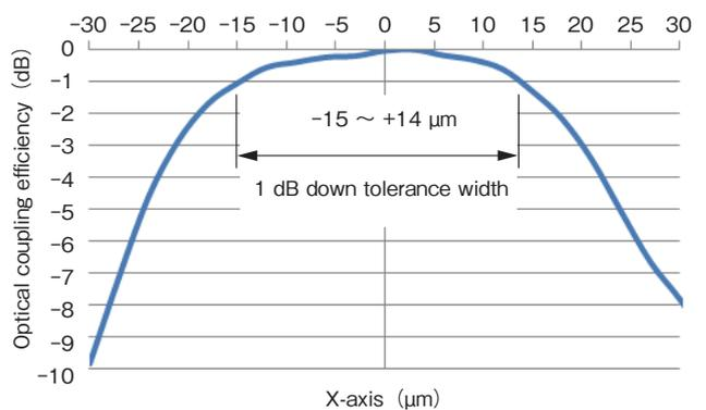
Figure 10 Positional tolerance.
