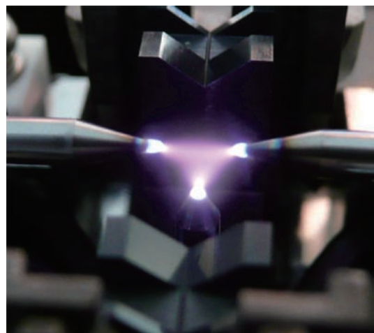
Figure 8 Appearance of 3-electrode arc discharge.
