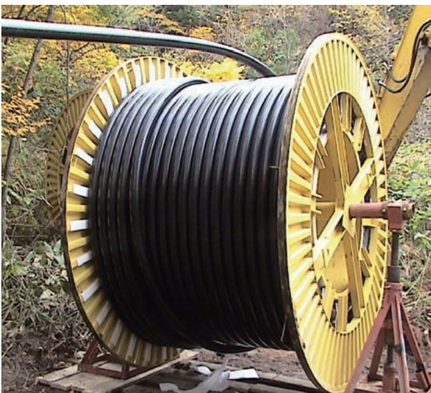
Figure 3 Supply in coil configuration (AQX-V).
