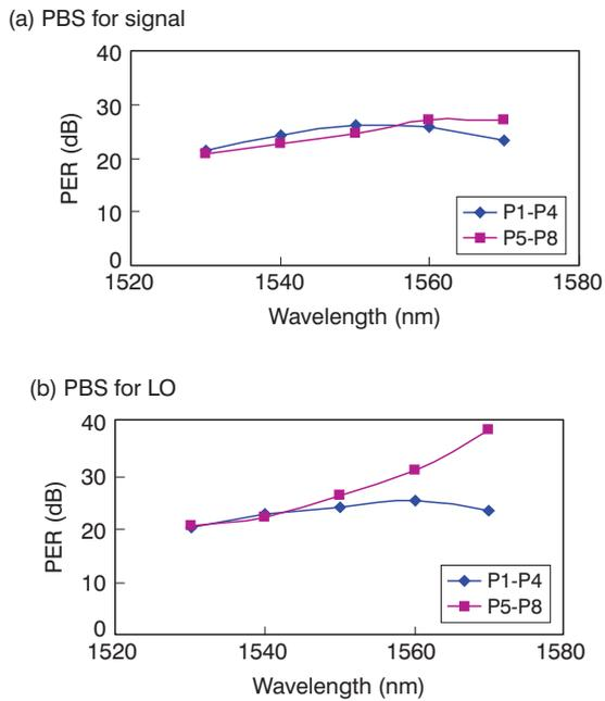
**Figure 9** The polarization extinction ratio of PBSs for (a) the signal and (b) the LO.
