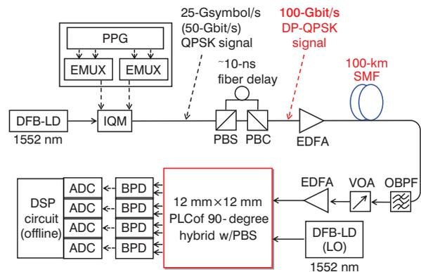
**Figure 11** The setup for a 100-Gbit/s DP-QPSK signal transmission experiment.
