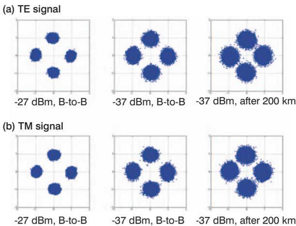
**Figure 4** The constellation maps of back-to-back (B-to-B) and transmitted DP-QPSK signals.
