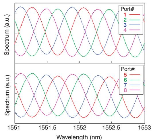
**Figure 2** The interference patterns of MZIs comprising the integrated coherent mixers.
