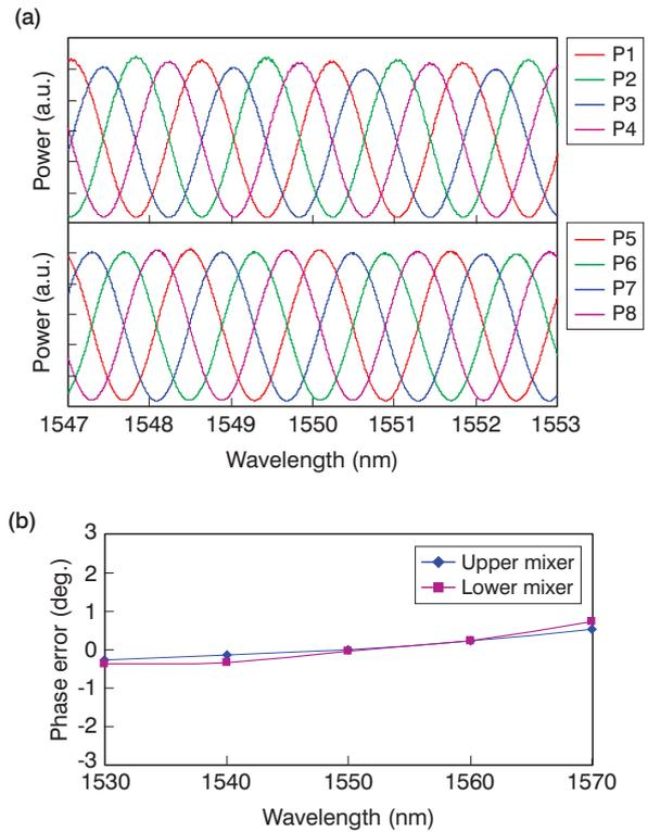
**Figure 10** The phase characteristics for the upper and lower mixers in the chip
