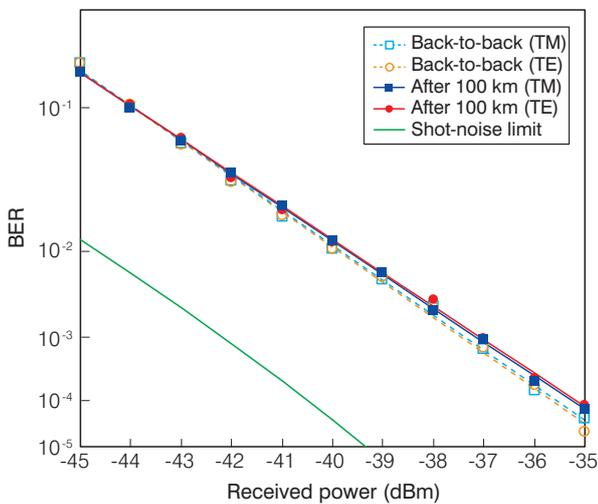
**Figure 13** The BER characteristics of 100-Gbit/s DP-QPSK signals.
