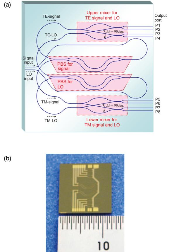
**Figure 7** (a) The schematic diagram of the proposed circuit layout with a folded configuration, and (b) picture of the fabricated PLC-chip.
