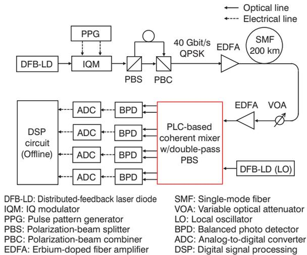
**Figure 3** The setup for the 40-Gbit/s DP-QPSK signal transmission experiment.
