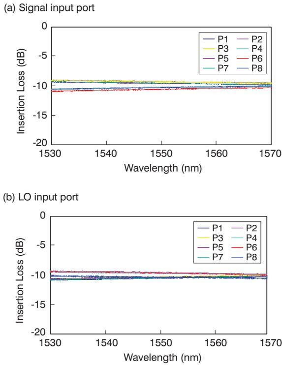
**Figure 8** The insertion loss from input ports for (a) the signal and (b) the LO to output ports P1-P8.
