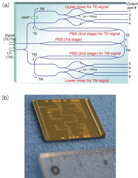
**Figure 1** (a) Schematic diagram of the proposed double-pass PBS-integrated coherent mixer based on PLC, and (b) picture of a fabricated PLC-chip.
