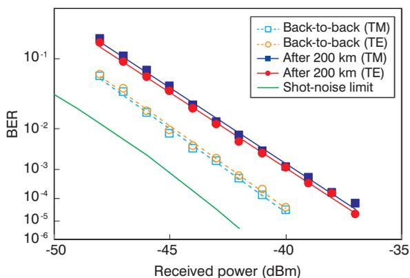
**Figure 5** BER characteristics of 40-Gbit/s DP-QPSK signals.
