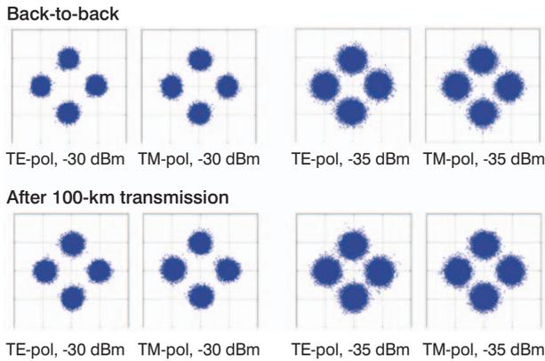
**Figure 12** The constellation maps of a back-to-back (B-to-B) and a transmitted DP-QPSK signals.
