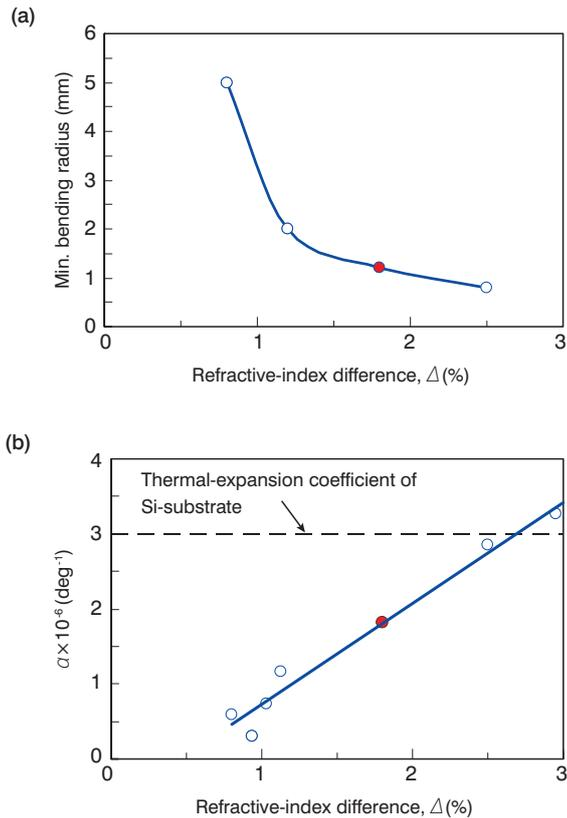
**Figure 6** (a) A minimum bending radius and (b) a thermal-expansion coefficient of the silica-based PLC vs.  $\Delta$ .
