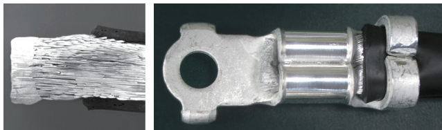
Figure 3 Ultrasonic soldered aluminum wire and crimping.
