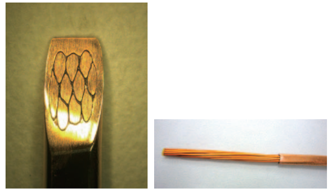
Figure 10 Usage example of enatube (cross section and profile).
