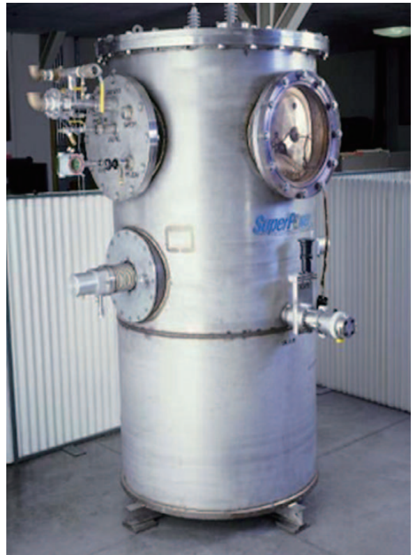
Figure 12 SFCL with 2G HTS wires developed by SuperPower Inc.
