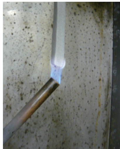
Figure 7 Vertical flame test (UL-94).
