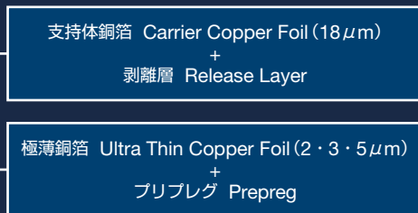
支持体銅箔付き極薄銅箔外観 Appearance of Ultra Thin Copper Foil with Carrier
