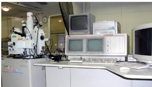
EPMA: Electron Probe Micro-analyzer
