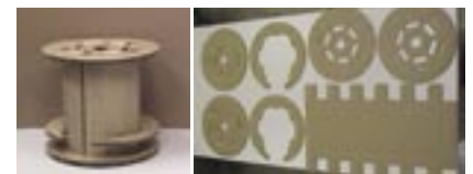
(Left) A paper bobbin using recycled corrugated cardboard for its frame (Right) A bobbin after taking to pieces
