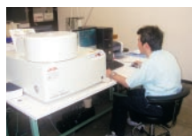
Measurement using fluorescent X-ray analysis
