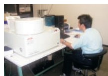
Measurement using fluorescent X-ray analysis
