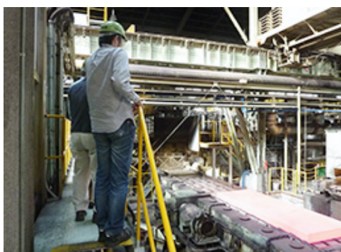
Copper rolling plant (A close-up look at the hot-rolling process)
