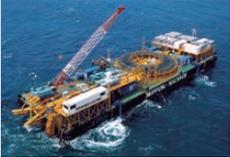
Submarine transmission cables and installation
