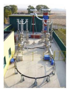
30m 275kV superconducting cable verification test (Shenyang)
