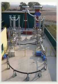
High-temperature super-conducting power cables
