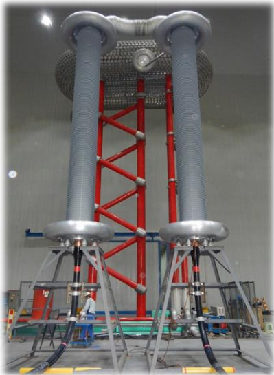
Type testing of a DC525kV cable system
