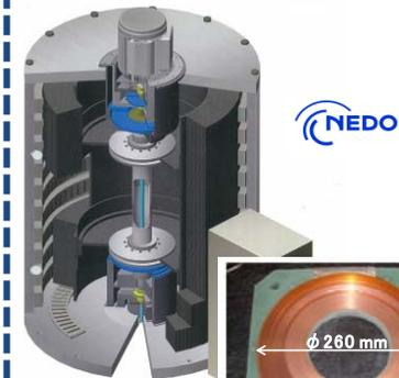
Superconducting magnet for next-generation flywheel storage system
