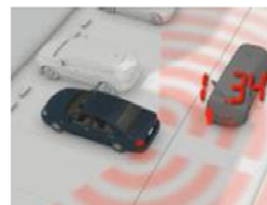
Proximity detection driving a car in reverse
