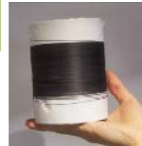
Succeed to make Jacket CNT wire sample
