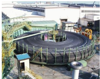
Turntable for winding the cable
