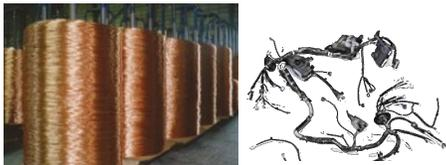
Conductor substrate for wire harnesses (copper, aluminum)
