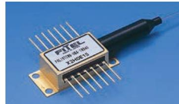
Contributed to advances in high volume communications through wavelength multiplexing technology (mass production of a 1480nm laser light source)
