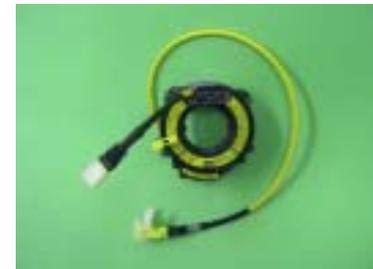
Steering roll connector for automotive air-bag
