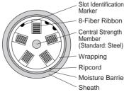
Marker 8-Fiber Ribbon Central Strength Member (Standard: Steel) Wrapping Ripcord Moisture Barrier Sheath
