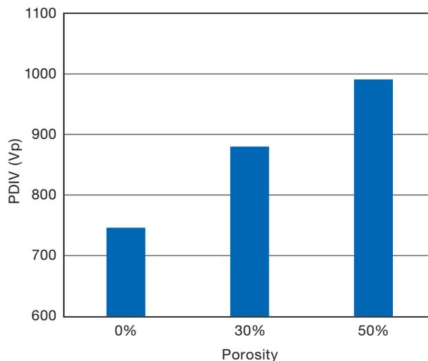
Figure 4 The PDIV as a function of porosity.
