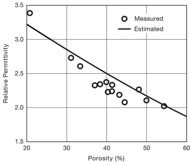
**Figure 2** Relative permittivity of PAI (Poly Amide Imide) as a function of porosity.
