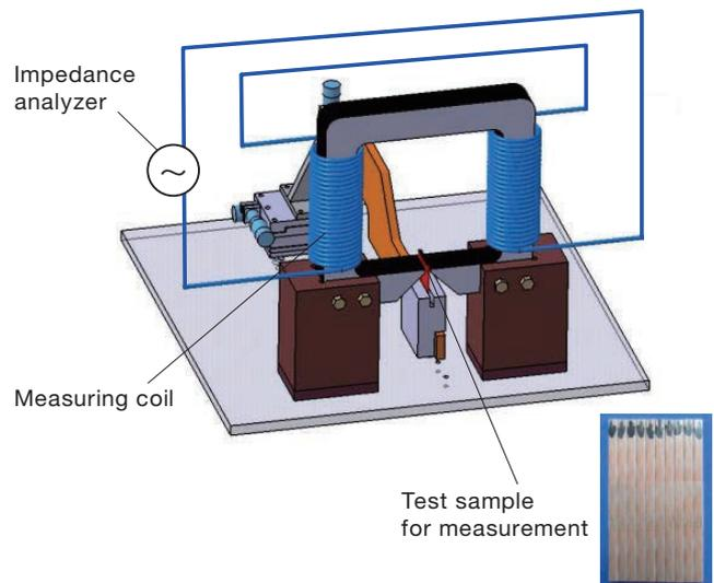
**Figure 9** A sketch of the measuring device of the eddy loss in a conductor.
