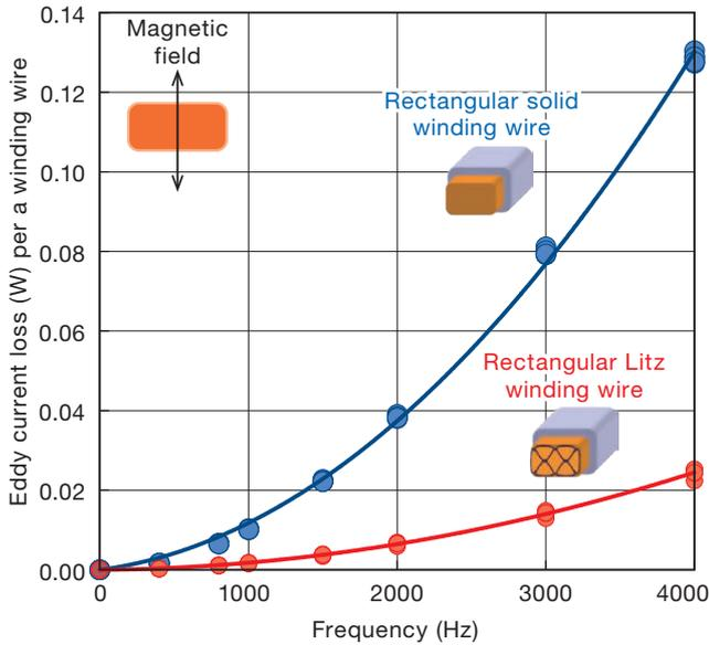
Figure 10 The comparison of the eddy current loss measured in a conductor of a solid winding wire and that of a Litz winding wire.
