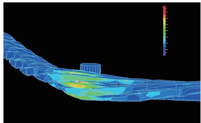
Figure 12 A result of an FEM analysis of bending the segmented conductors.
