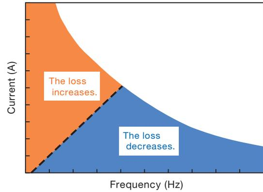
Figure 11 The decrease / increase of the copper loss of the segmented conductor winding wire on a plane by frequencies and currents.
