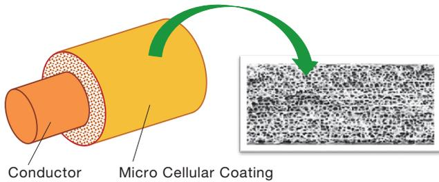
**Figure 1** A sketch of the developed winding wire coated with the micro cellular film.
