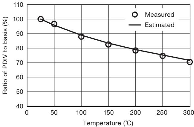
Figure 5 The temperature dependence of the PDIV.
