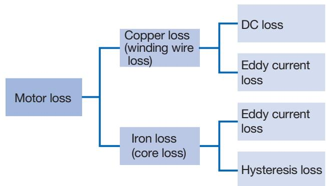
Figure 7 The classification of motor losses.
