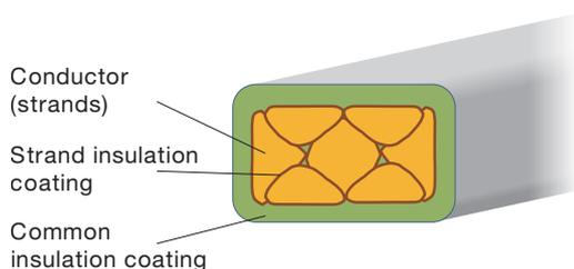
**Figure 8** The structure of the segmented conductor winding wire.
