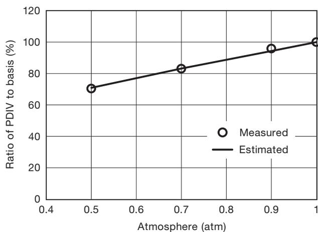
Figure 6 The atmospheric pressure dependence of the PDIV.
