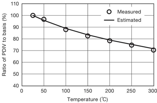
Figure 5 The temperature dependence of the PDIV.
