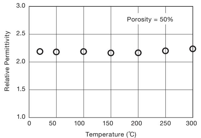
**Figure 3** The Temperature dependence of the relative permittivity.
