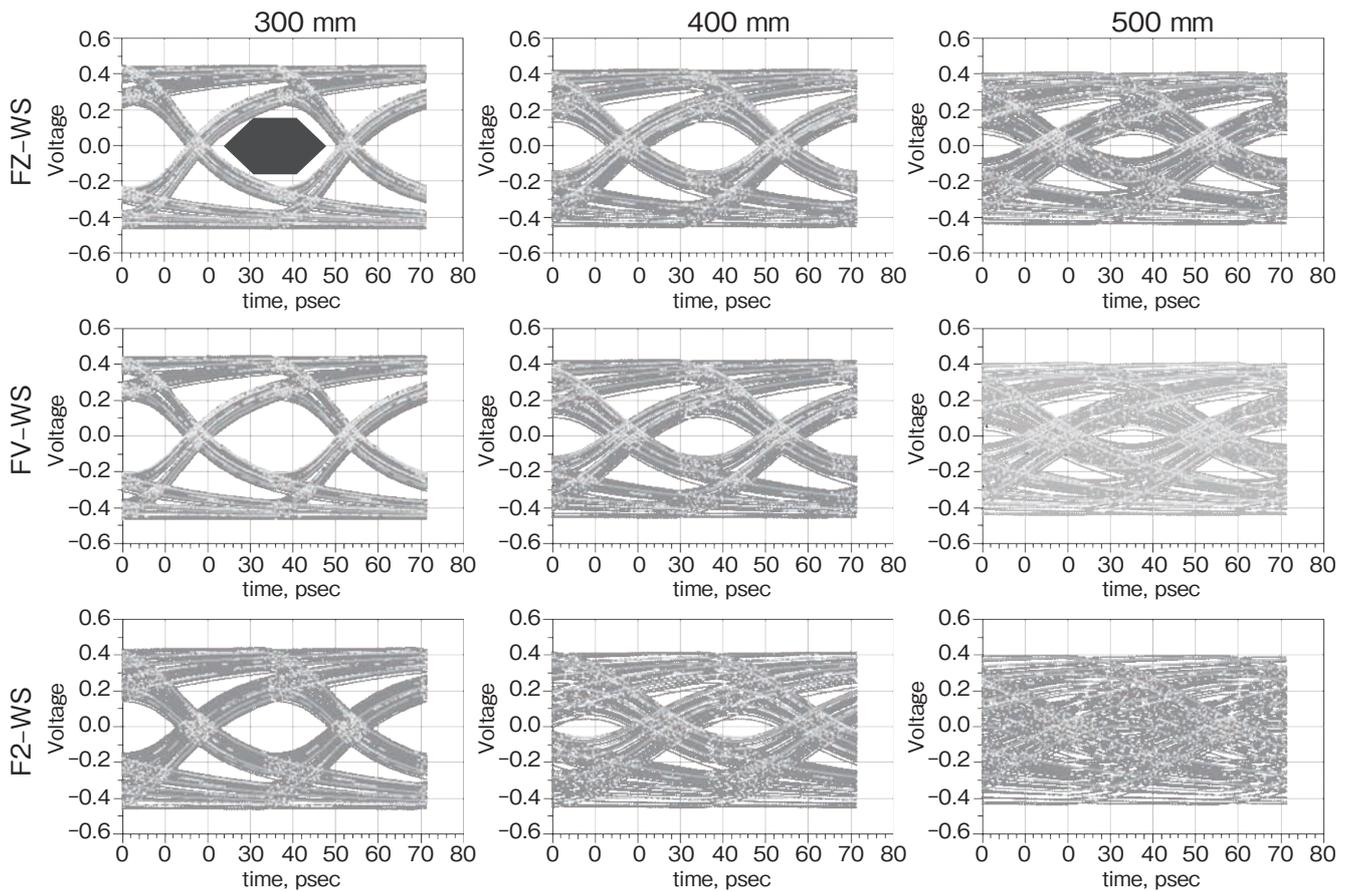
Figure 11 28 Gbps high-speed digital simulation results.
