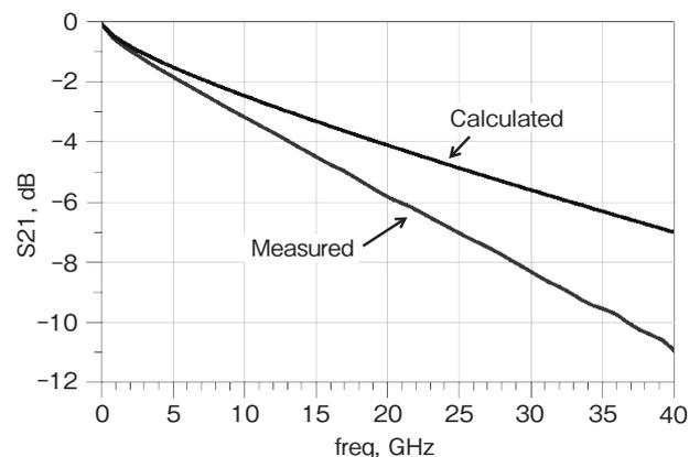
Figure 7 Comparison of the calculated and the measured attenuations of the strip-line transmission line.
