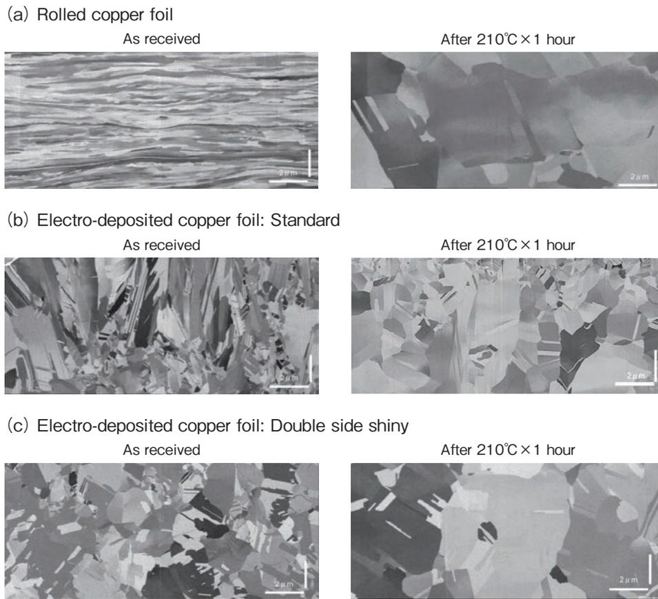
Figure 5 X-section crystal structures of copper foils.
