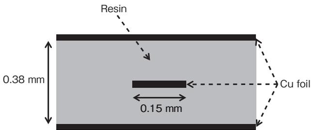
Figure 8 X-section of the PCB for S-parameter measurement.
