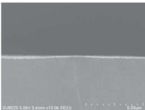
**Figure 4 (a) Matt surface of double side shiny foil: Untreated.**
