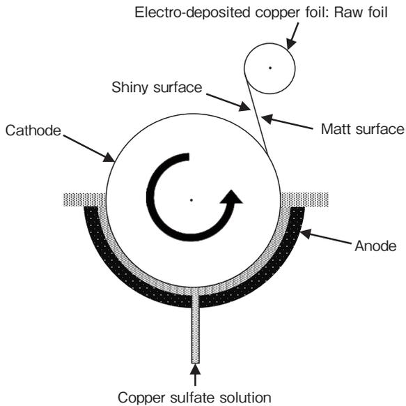
**Figure 1** A schematic X-section of the manufacturing equipment.
