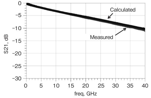
Figure 10 Comparison of values calculated and measured for the electro-deposited copper foil FV-WS.
