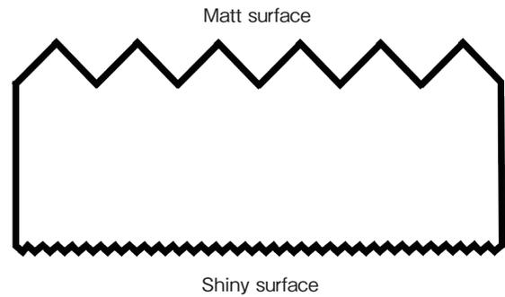
**Figure 2 (a)** A schematic X-section of a standard foil.
