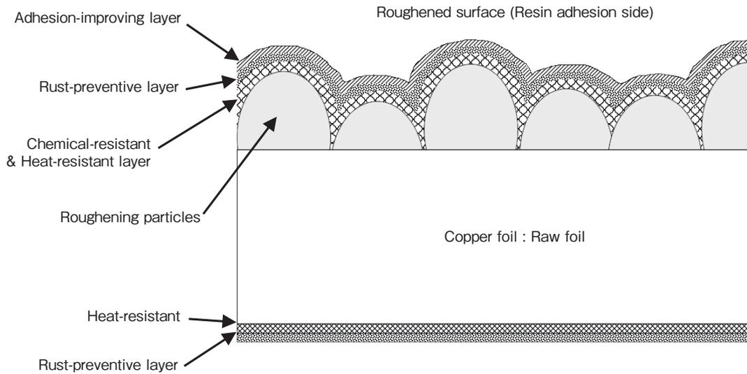
**Figure 3 A schematic X-section of the copper foil for PCB.**
