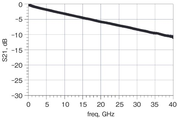
Figure 9 Measured S-parameter S21.
