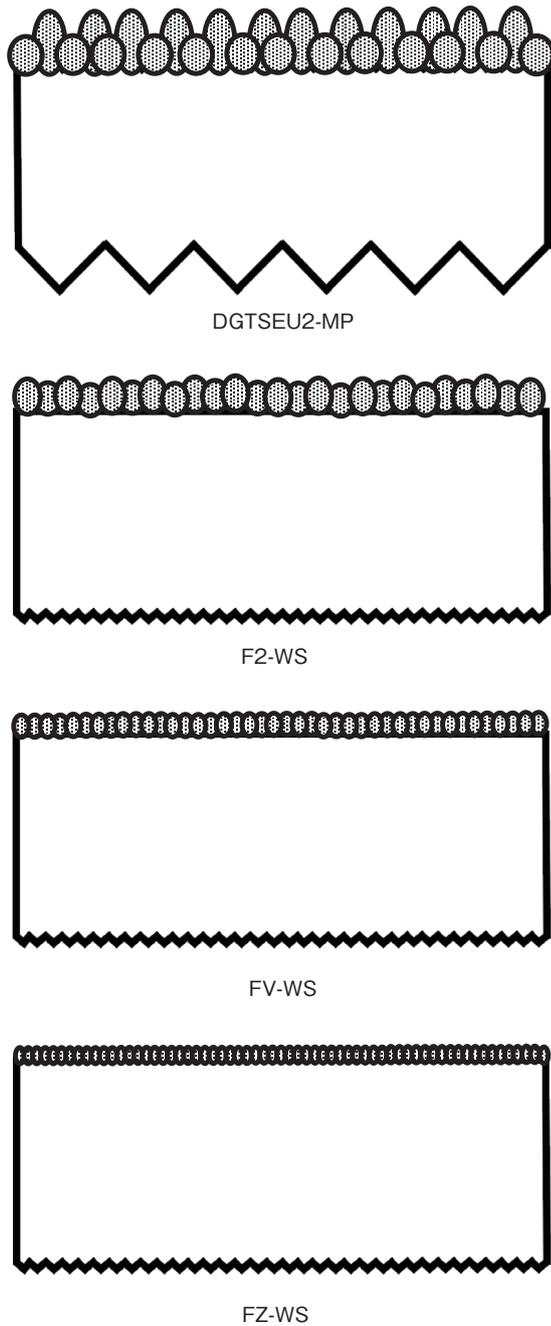
Figure 6 Schematic X-sections of high-frequency compatible products.
