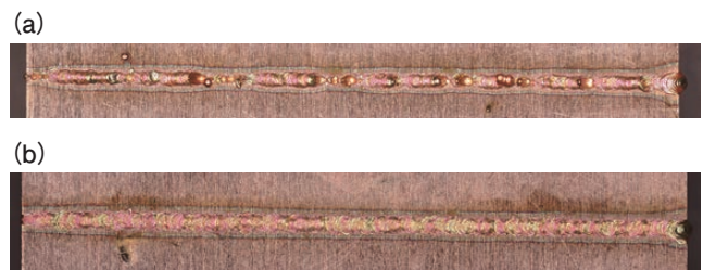
Figure 10 Images of the beads on the pure copper sheet. (a) With the conventional single focused spot (b) With the beam mode control technology
