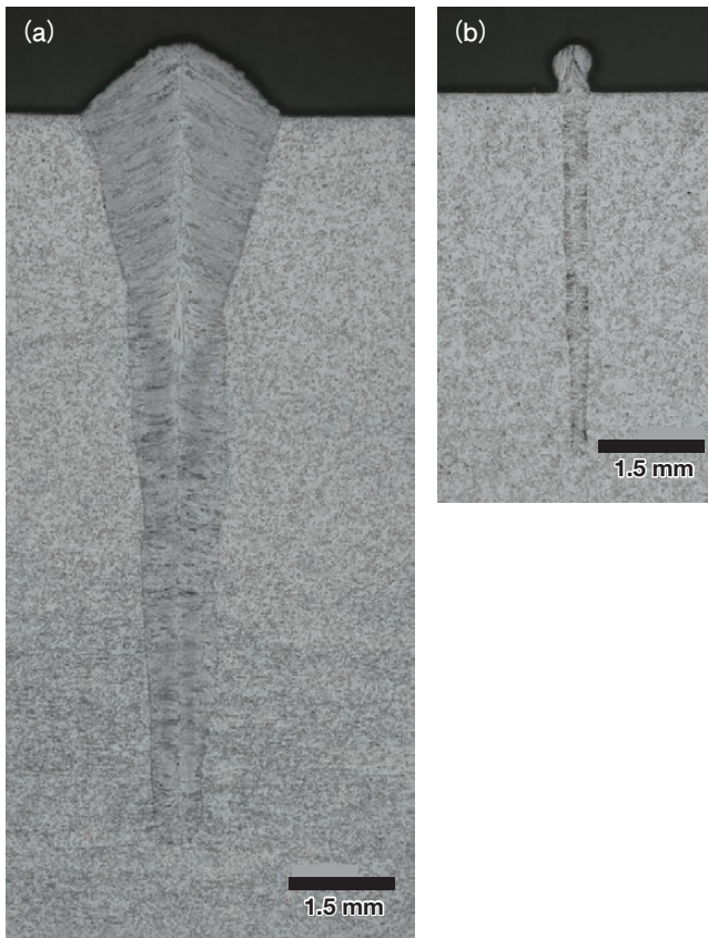
Figure 5 Cross-sectional view of the steel processed with a 6 kW multi-mode fiber laser. (a) 1 m/min (b) 10 m/min
