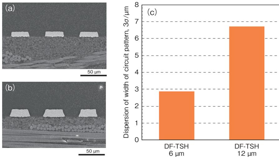
Figure 2 Fine pattern formation on L&S = 30/30 μm by the Subtractive process.
