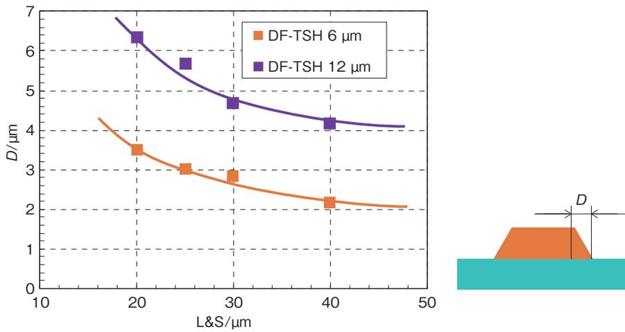
Figure 1 Effect of the copper foil thickness for pattern trailing length  $D$  by the Subtractive process.
