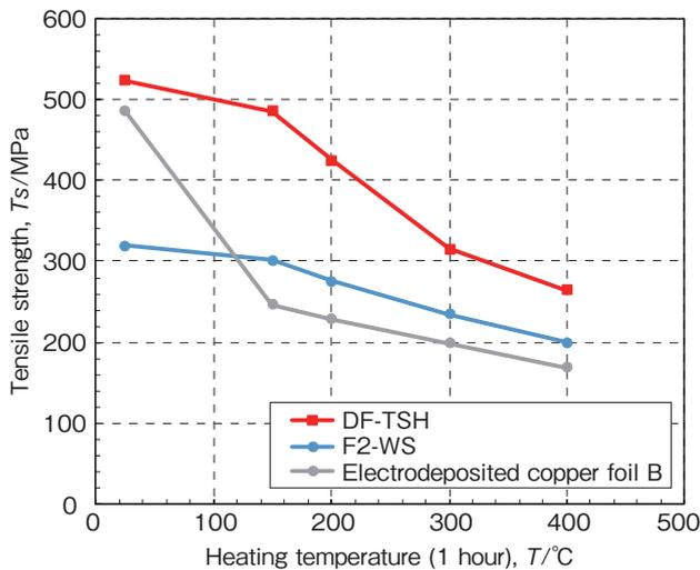
**Figure 3 Thermal stability of DF-TSH compared with other electrodeposited copper foils.**
