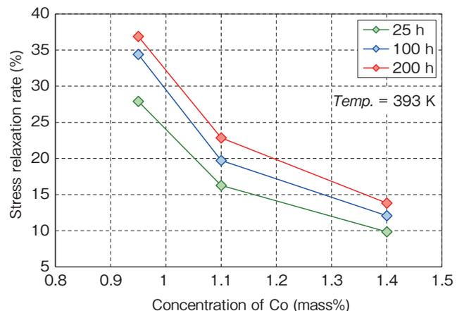
Figure 6 Changes in the stress relaxation rates after testing vs the concentration of Co.
