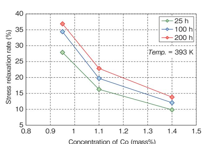
Figure 6 Changes in the stress relaxation rates after testing vs the concentration of Co.
