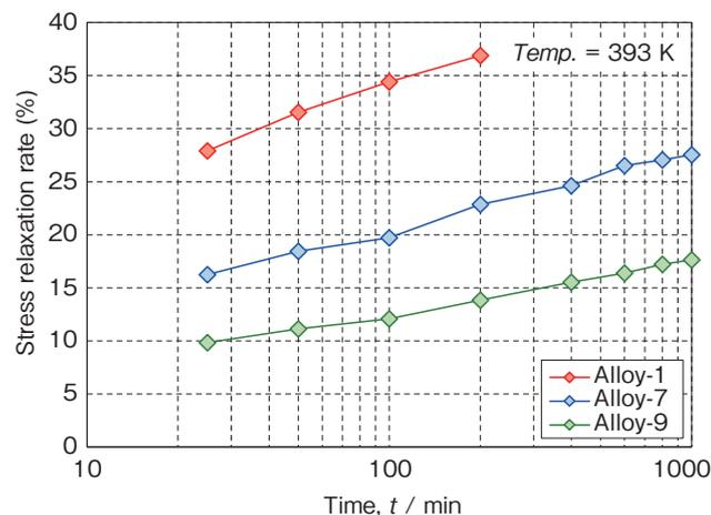
Figure 5 Changes in the stress relaxation rates of the Cu-Co-Si alloys vs the testing time.
