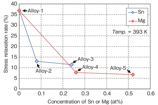
**Figure 9** Changes in the stress relaxation rates after testing for 200 hours vs the Sn or Mg concentrations.
