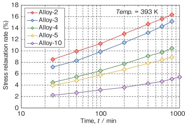
**Figure 8** Changes in the stress relaxation rates of the Cu-Co-Si-Sn-Mg alloys vs the testing time.
