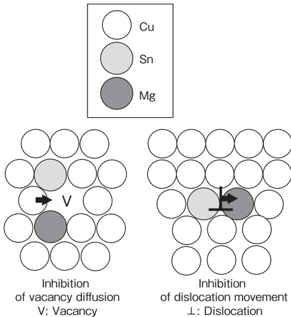
**Figure 10** Schematic illustration of the inhibition of vacancy diffusion and dislocation movement.
