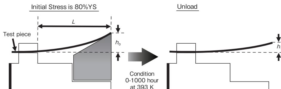
**Figure 1 Schematic illustration of the stress relaxation test.**
