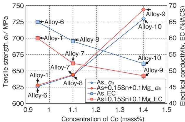
**Figure 2** Changes in the tensile strengths and the electrical conductivities of the Alloy-1, -6, -7, -8, -9 and -10 after annealing at 673 K vs the Co concentration.
