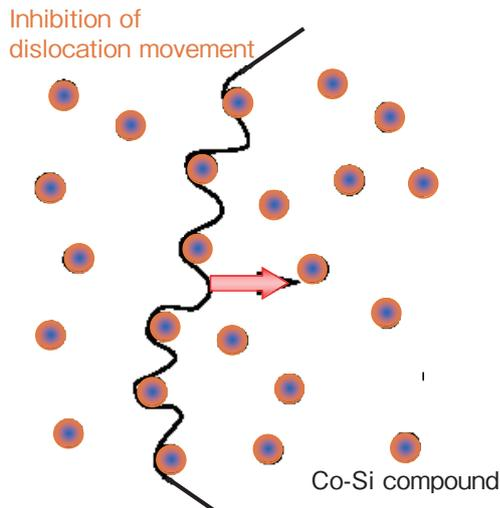
**Figure 7** Schematic illustration of the dislocation movement inhibited by the Co-Si compounds.
