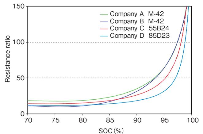
Figure 4 Relation between  $R_{ratio}$  and SOC.
