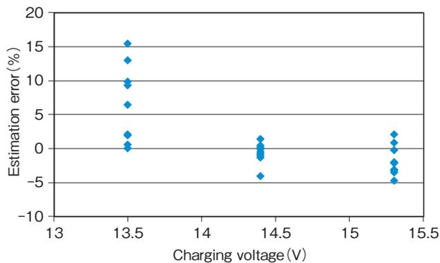
**Figure 8** Error of the full charge detection when ignoring the charging voltage.
