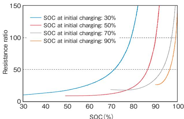
**Figure 6** Difference of the relation between the resistance ratio and the SOC caused by difference of SOC at initial charging.
