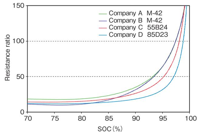
Figure 4 Relation between  $R_{ratio}$  and SOC.
