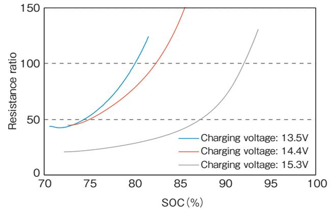
**Figure 7** Difference of the relation between the resistance ratio and the SOC caused by difference of charging voltage.
