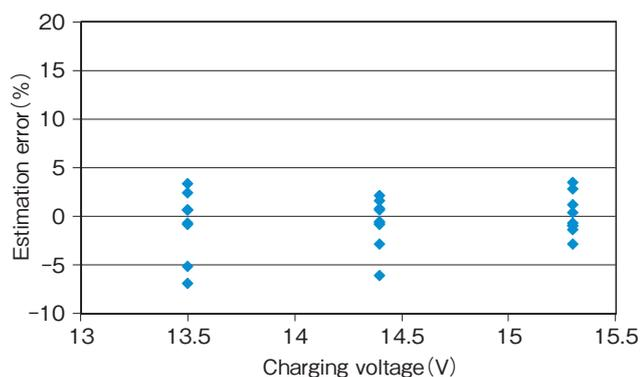
**Figure 11** Error of the estimated full charge when considering the charging voltage.
