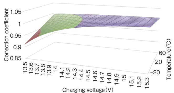
**Figure 10** A 3-dimensional curved surface of correction coefficient vs. charging voltage and temperature.
