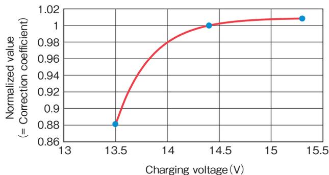
**Figure 9** Normalized SOC at full charge detection against various charging voltage.
