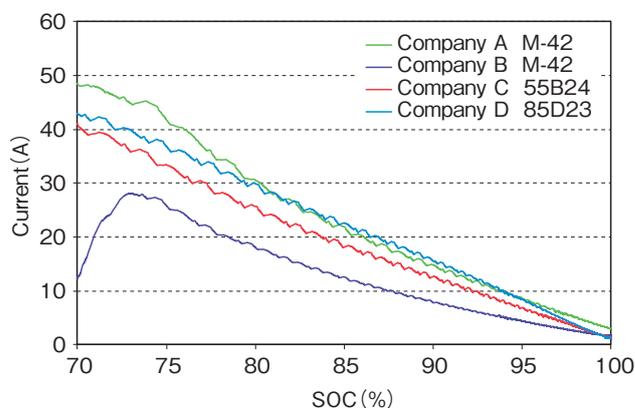
Figure 2 Relation between the charging current and the SOC.
