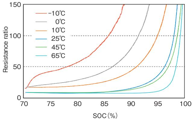
**Figure 5** Difference of the relation between the resistance ratio and the SOC caused by the different temperature.
