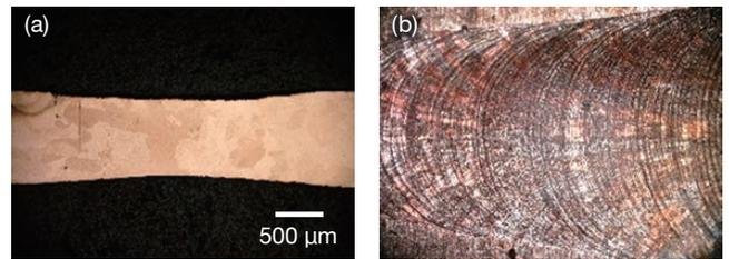
**Figure 14** Bead-on welding experiment results using a multi-beam processing head (output 1,000 W). (a) Cross-sectional photograph in the direction perpendicular to the scanning direction of the laser focused spot (b) Surface photograph
