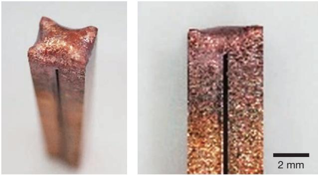
**Figure 11** High-speed welding for a pure copper square wire using a hybrid laser system that combines a blue diode laser and a near-infrared fiber laser.
