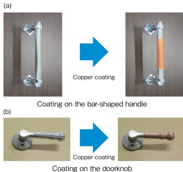
**Figure 5** High-speed and precise coating of copper using a blue diode laser. (a) Coating on the bar-shaped handles and (b) Coating on the doorknobs
