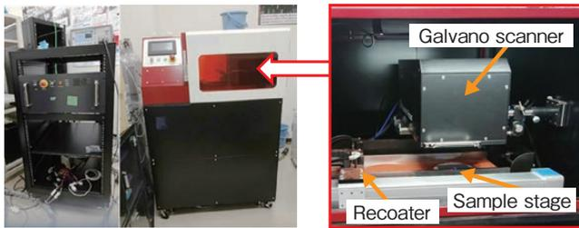
**Figure 7** External appearance photograph of a SLM method 3D printer equipped with a blue diode laser.
