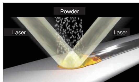
Figure 3 LMD using a multi-beam method.
