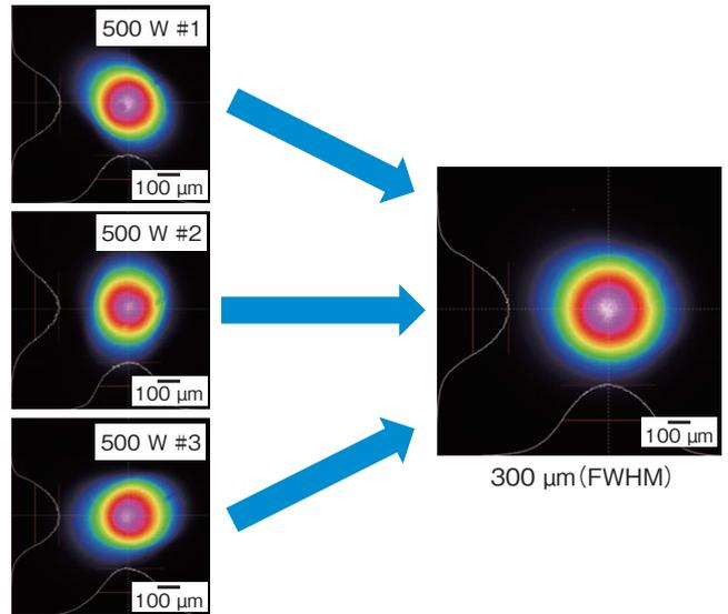
**Figure 13** Beam profile superimposed with three 500 W blue diode lasers.
