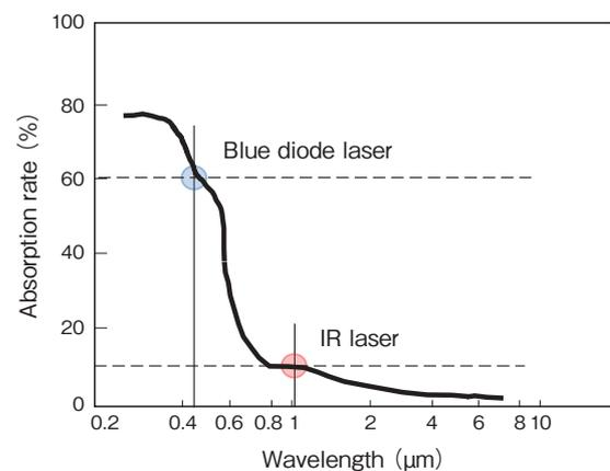
Figure 2 Light absorption rate for copper.
