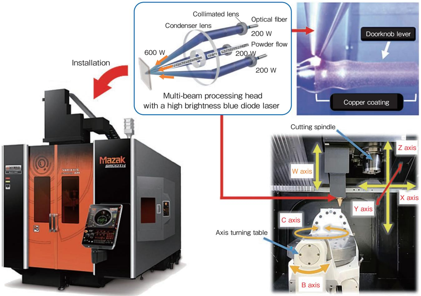
**Figure 4** Multi-beam processing head equipped with three 200 W blue diode lasers and hybrid multi-tasking processing machine with a processing head.
