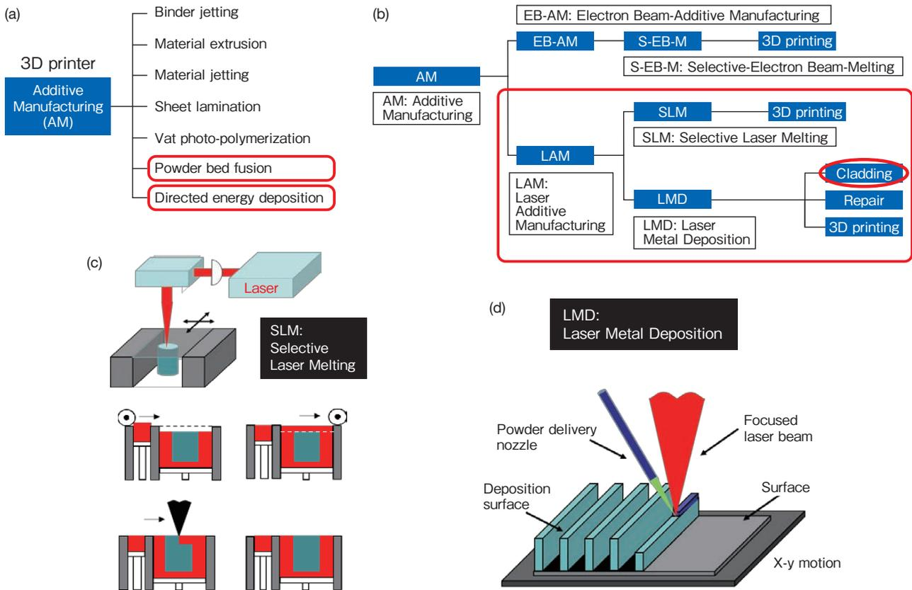
**Figure 1** (a) Additive Manufacturing (AM) and 7 categories, (b) Laser Additive Manufacturing (LAM: AM using a laser.), (c) Selective Laser Melting (SLM: Powder bed fusion method using a laser.), (d) Laser Metal Deposition (LMD: Directed energy deposition method using a laser.)
