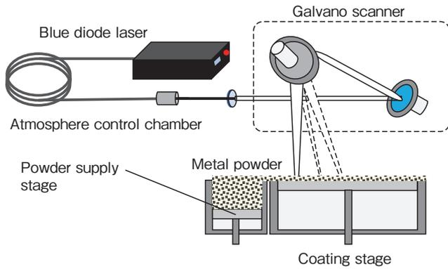
**Figure 6** Schematic diagram of a SLM method 3D printer equipped with a blue diode laser.
