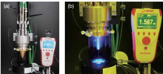
**Figure 12** Multi-beam processing head using three 500 W blue diode lasers has been developed. (a) Processing head (b) Laser output
