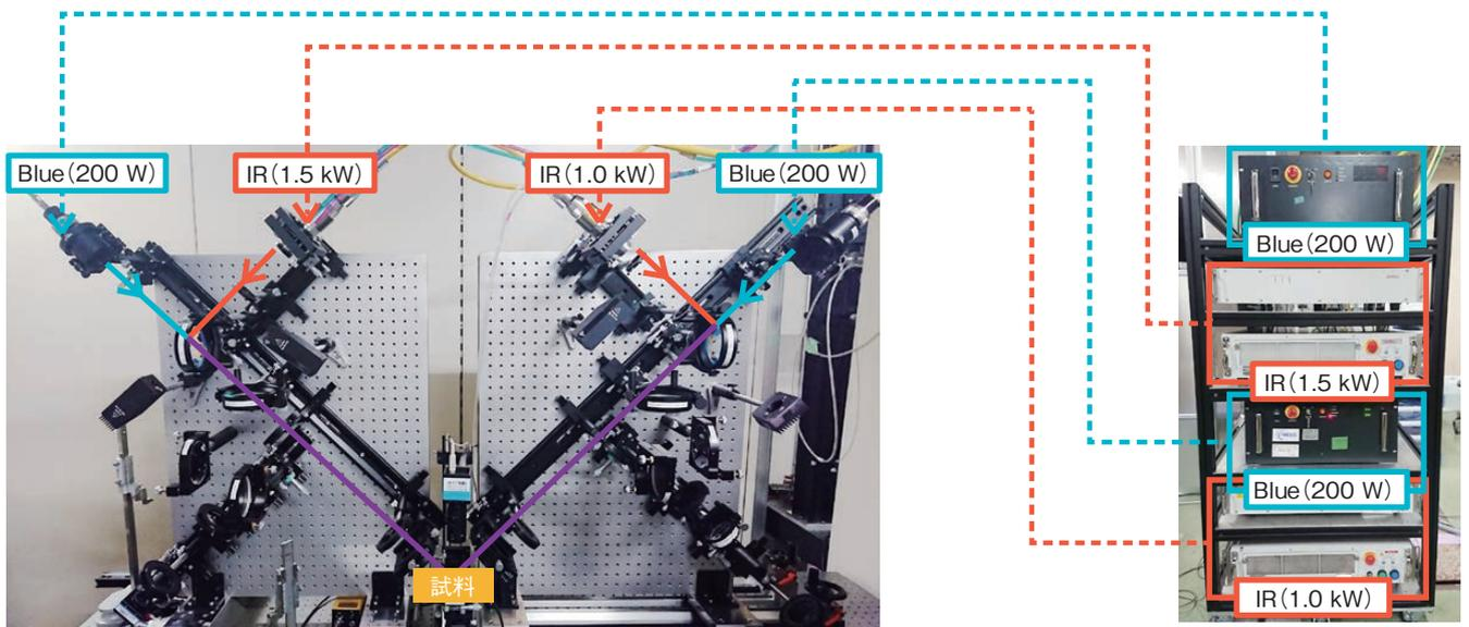
**Figure 10** Setup photograph of a hybrid laser irradiation optical system that combines a blue diode laser and a near-infrared fiber laser.
