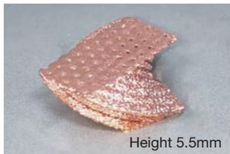
**Figure 8** Pure copper laminated molding using a SLM method 3D printer equipped with a blue diode laser.
