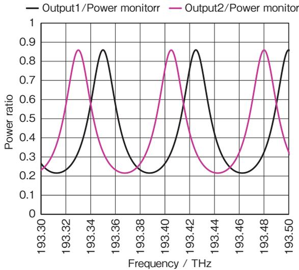
Figure 5 Output characteristics of the PLC.
