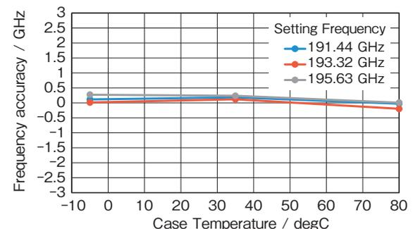
Figure 9 Wavelength locking characteristics.
