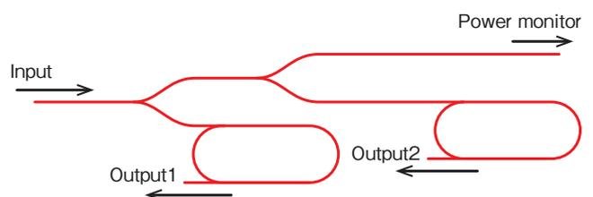
Figure 4 Optical circuit diagram of the PLC.
