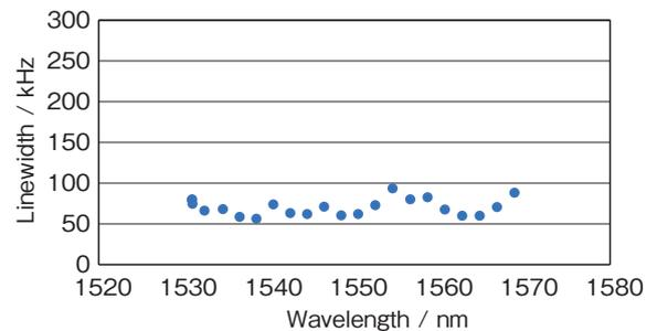
Figure 8 Spectral linewidth characteristics.
