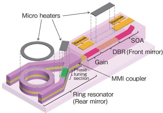
Figure 1 Structure of the wavelength tunable laser chip.
