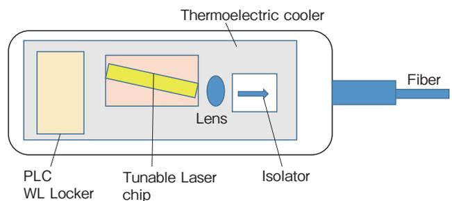
Figure 3 Structure of the laser module.
