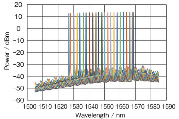
Figure 7 Oscillation spectrum characteristics.
