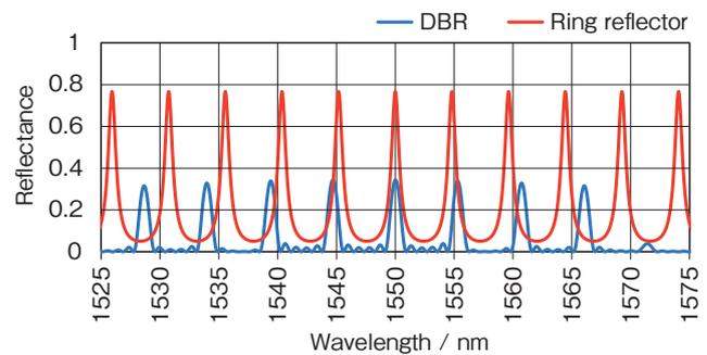
(a) Calculation example of the reflection spectrum of a DBR and a ring reflector.
