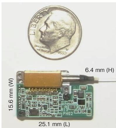
Figure 6 Picture of the developed Nano-ITLA.
