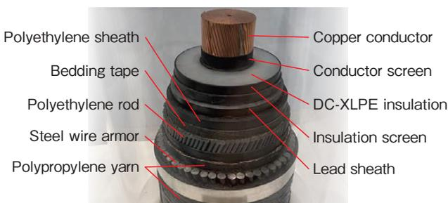
**Figure 10 DC 525 kV 1800 mm<sup>2</sup> submarine power cable.**
