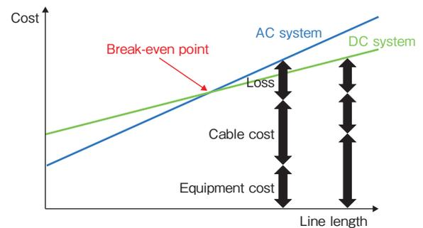
Figure 8 Cost comparison between AC and DC systems.
