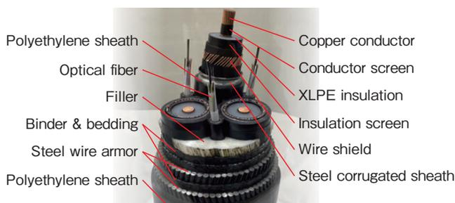
Figure 6 AC 66 kV 100 mm<sup>2</sup> dynamic cable.
