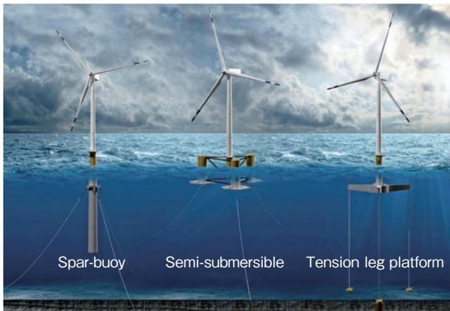
Figure 7 Example of a floating wind turbine.<sup>9)</sup>
