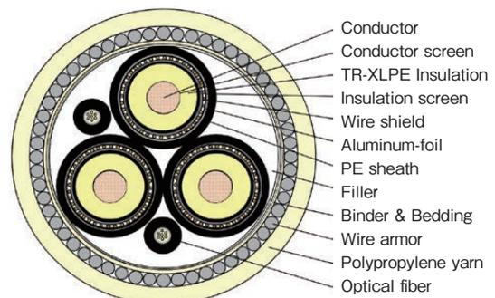
Figure 3 Cross section of semi-dry structured submarine power cable.
