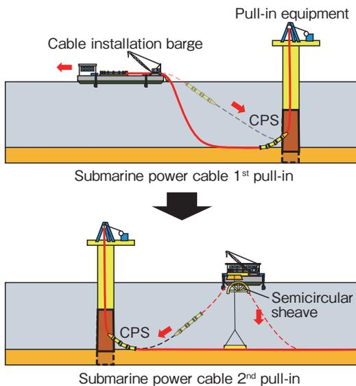
Figure 12 Example of a submarine power cable installation procedure for fixed wind power generation.
