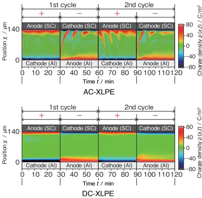
**Figure 9 Comparison of space charge characteristics between AC and DC materials.**
