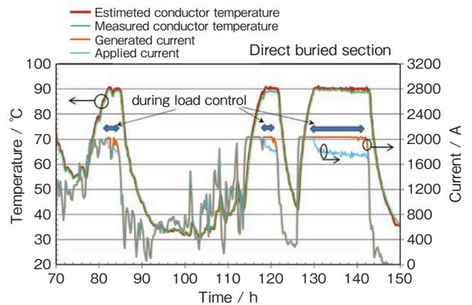
(1) Conductor temperature of cable and applied current.
