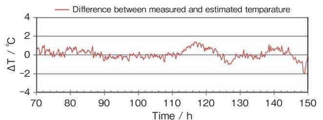
(2) Error of estimated conductor temperature.
