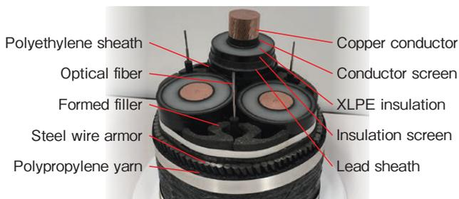
Figure 4 AC 275 kV 1400 mm<sup>2</sup> submarine power cable.
