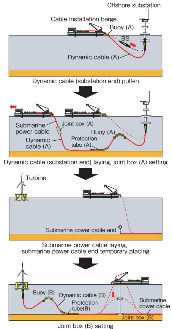
Figure 13 Example of dynamic cable installation procedure.
