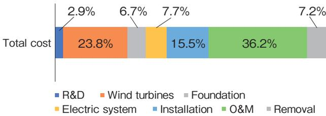
Figure 14 Cost structure of the offshore wind industry (Fixed wind power generation).<sup>14)</sup>
