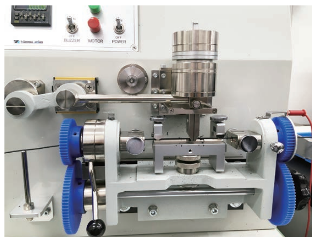
Figure 3 The scrape testing machine for wear resistance.
