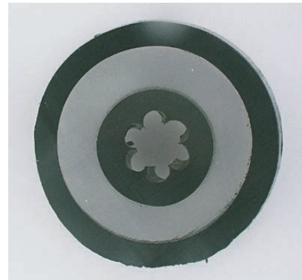
Figure 12 Cross-section of a miniature cable (the copper strands in the center are falling out).
