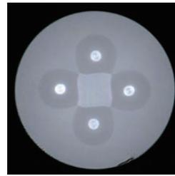
Figure 9 Cross-sectional picture of MCF fabricated using the modified cross-shaped cylinder.
