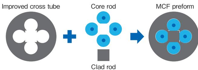
Figure 6 Design of MCF preform using the modified cross-shaped cylinder.
