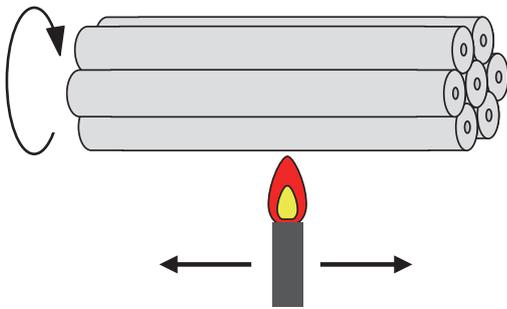
**Figure 3** Schematic illustration of the over-cladding bundled rods method.
