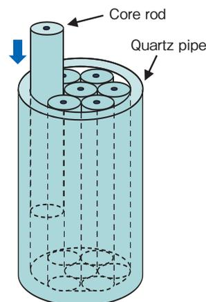
Figure 2 Structure of MCF preform using the stack and draw method.
