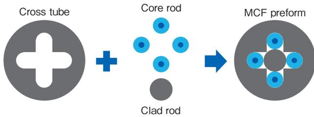
Figure 4 Design of MCF preform using the cross-shaped cylinder.
