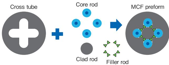
Figure 5 Design of MCF preform using the cross-shaped cylinder with a low gap ratio.
