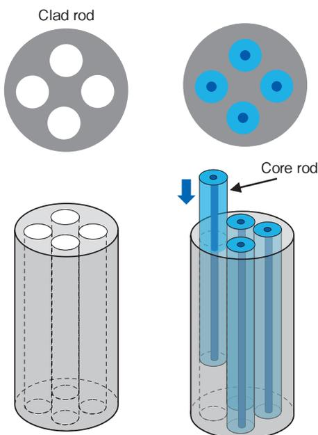
Figure 1 Structure of MCF preform using the drilling method.
