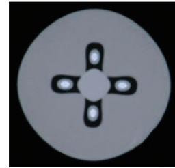
Figure 7 Cross-sectional picture of MCF fabricated using the cross-shaped cylinder.
