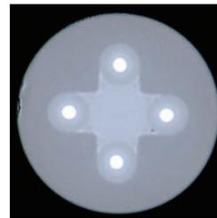
Figure 8 Cross-sectional picture of MCF fabricated using the cross-shaped cylinder with filler cladding rods.
