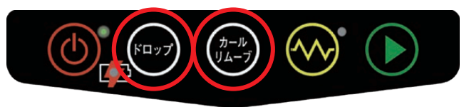
Figure 7 A button for splicing the drop cable and a button for removing the fiber curl.
