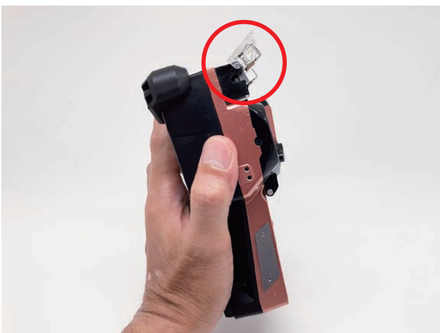
Figure 4 Rocker type heater lid.
