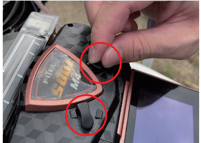
Figure 5 Optical fiber position correcting levers.
