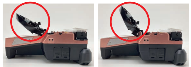
Figure 6 Windshield with adjustable opening angle.
