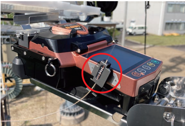
Figure 3 Optical fiber holder magnetic attraction plate.
