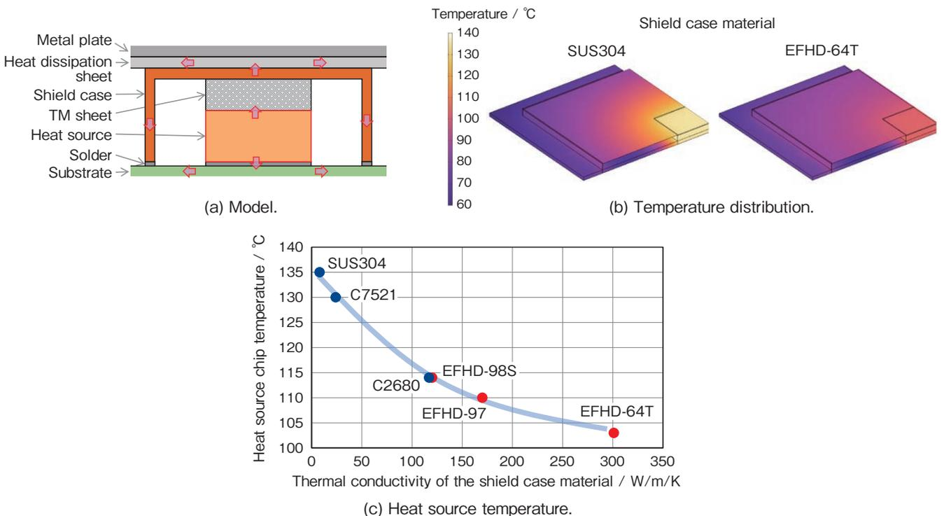
Figure 4 Heat dissipation simulation of the shield case.
