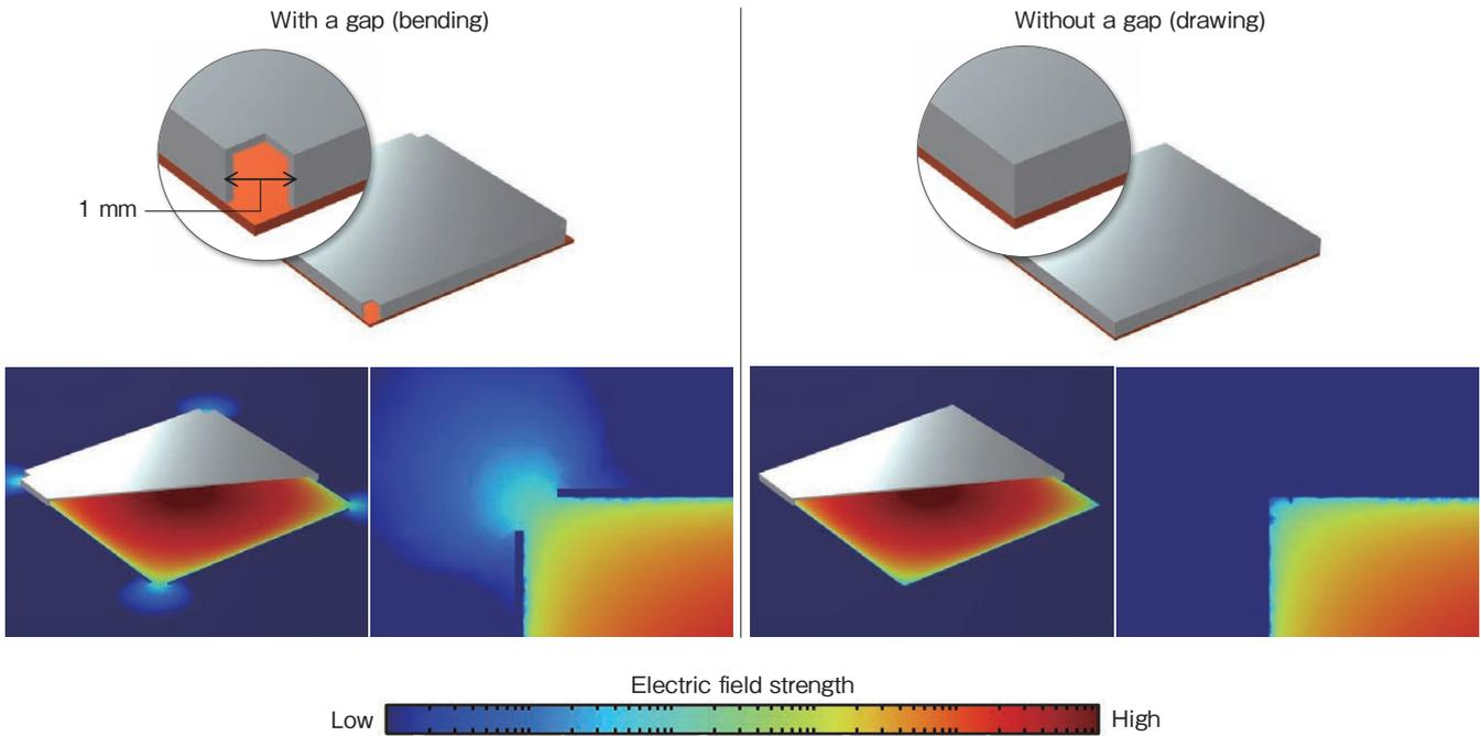
Figure 5 Electromagnetic wave shield simulation of the shield cases.
