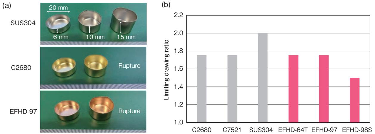
Figure 2 Drawability. (a) Appearance of the cylindrical drawn products, (b) Limiting drawing ratio.
