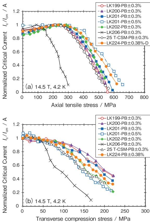
**Figure 7**  $I_c$  values normalized at the respective peak  $I_c$  values of the Cu-Nb reinforced Nb<sub>3</sub>Sn wire and the unreinforced Cu/Nb<sub>3</sub>Sn wire at 4.2 K and 14.5 T under tensile stress. (a) Under axial tensile stress. (b) Under transverse compressive stress.
