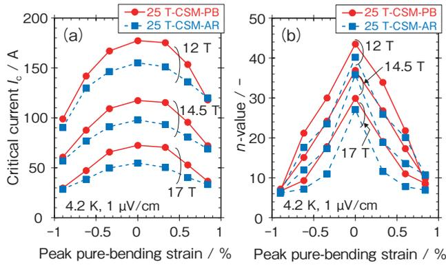
**Figure 5**  $I_c$  characteristics of the Cu-Nb/Nb<sub>3</sub>Sn wire for the 25 T-CSM against the peak pure-bending strain<sup>12)</sup>.
