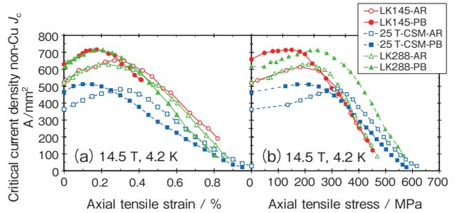
**Figure 9** Comparison of the critical current density characteristics in the non-Copper part at 14.5 T between the high critical current density round wires (LK145, LK288) and the 25 T-CSM wire under axial strain and axial stress<sup>(5), (13), (18)</sup>. (a) Axial tensile strain, (b) Axial tensile stress
