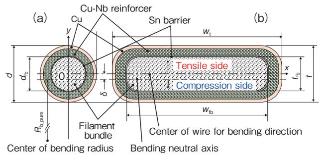
**Figure 6** Cross-sectional structure model of the wire for the analysis of the pure-bending strain effect on the  $I_c$  of the Cu-Nb/Nb<sub>3</sub>Sn wire<sup>17)</sup>. (a) round wire, (b) tape wire
