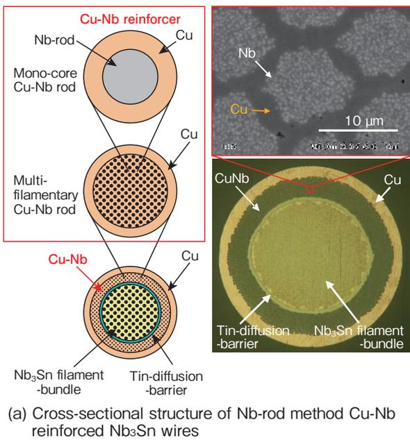
(a) Cross-sectional structure of Nb-rod method Cu-Nb reinforced Nb<sub>3</sub>Sn wires
