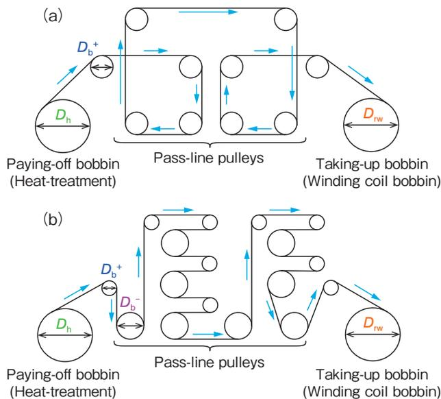
**Figure 3** Schematic diagram of the pass line for applying pre-bending strain; (a) forward bending, (b) bidirectional bending (forward and backward directions)<sup>(5)</sup>.
