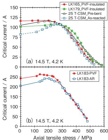
**Figure 10** Comparison of critical current characteristics under axial tensile stress of the Cu-Nb/Nb<sub>3</sub>Sn wire with PVF insulation coating and the wire without PVF coating<sup>14)</sup>. (a) Comparison of the PVF-coated wire K165, the LK179 and the 25 T-CSM wire, (b) Comparison of the PVF-coated wire LK183 and the uncoated wire LK183
