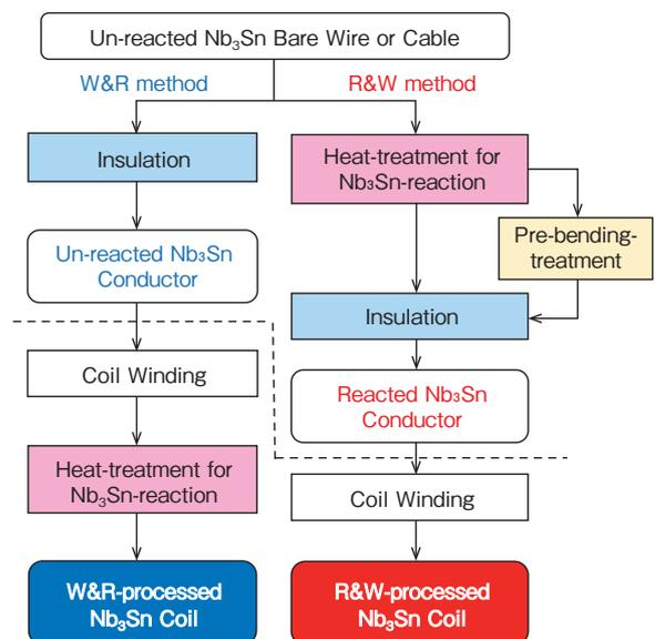
**Figure 2** Comparison of the Nb<sub>3</sub>Sn coil manufacturing flow between the W&R method and the R&W method.
