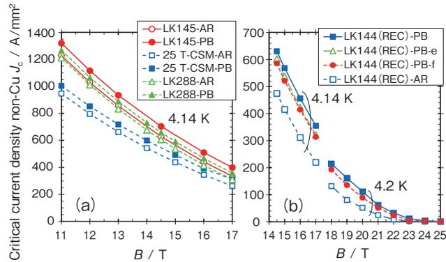
**Figure 8** Magnetic field dependence of the critical current density in the non-Copper part<sup>(5), (13), (18)</sup>. (a) round wire, (b) rectangular wire
