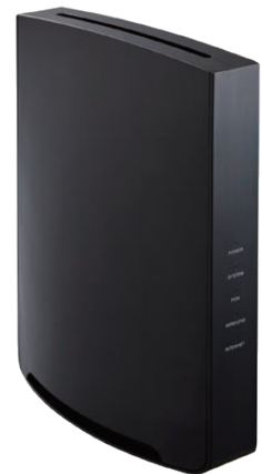
Figure 5 Picture of ONU AG30 with built-in broadband router.
