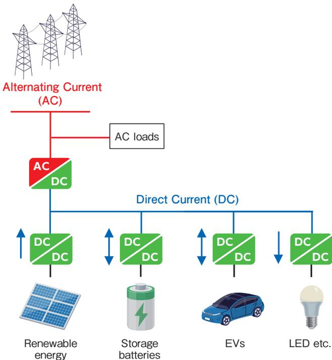
Figure 1 Schematic diagram of DC-MG.
