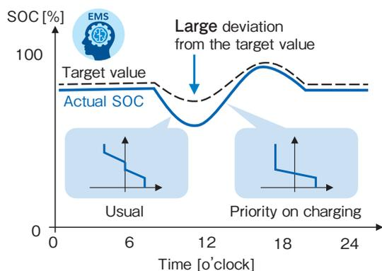
Figure 9 Schematic diagram of a SOC control.
