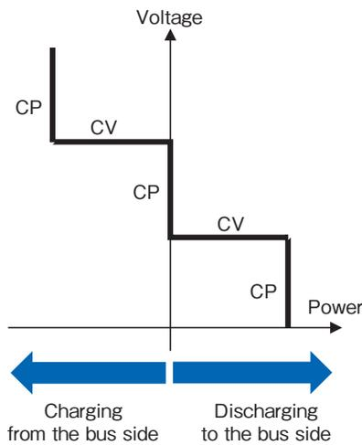
Figure 4 Voltage-margin control method.
