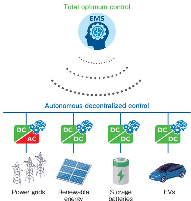
Figure 6 Schematic diagram of a hierarchical autonomous decentralized control.
