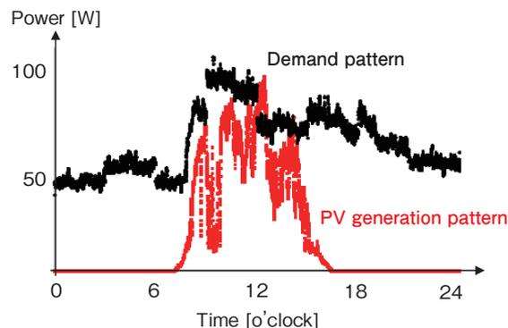
Figure 10 Patterns of demand and of a solar power generation.
