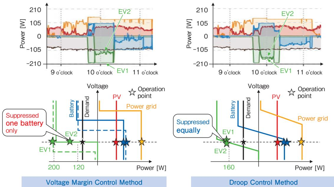
Figure 13 Comparison of Droop Control Method and Voltage Margin Control Method in EV charging control.
