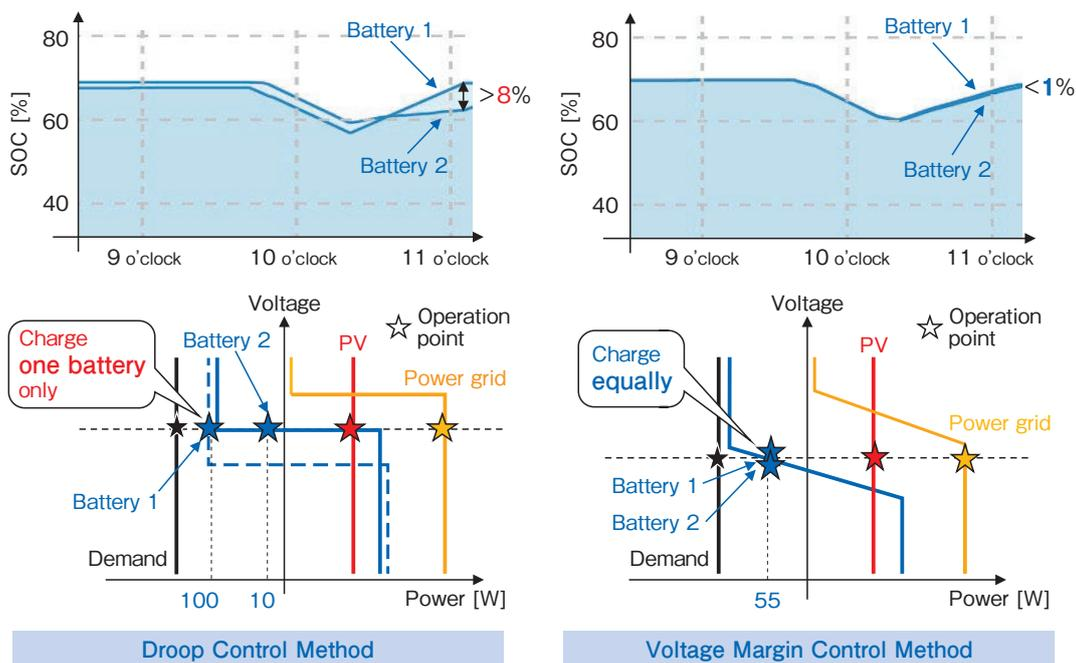
Figure 12 Comparison of the Droop Control Method and the Voltage Margin Control Method in battery charging.
