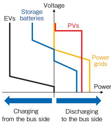
**Figure 7 Example of Droop function for each device.**
