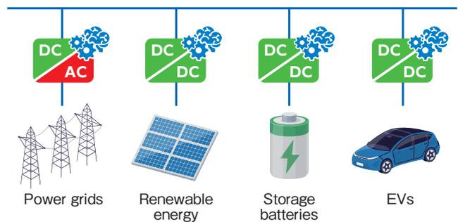
Figure 3 Schematic diagram of an autonomous decentralized control.
