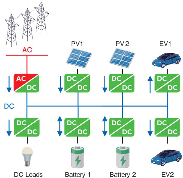
**Figure 8 Schematic diagram of the demonstration system.**
