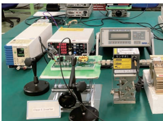
Figure 6 Developed class E inverter (size: 145 x 80 x 25 mm).
