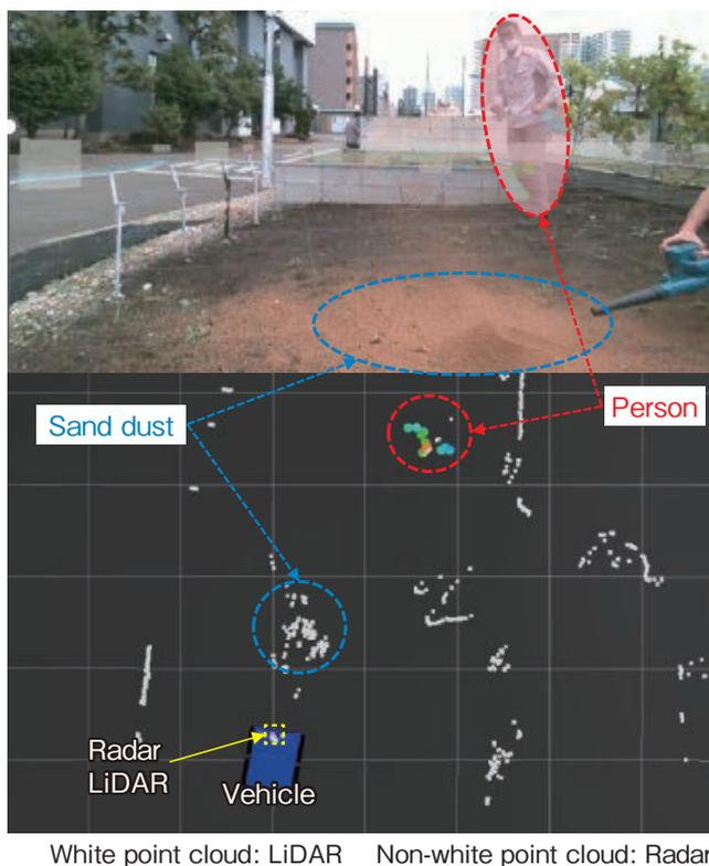
Figure 10 Comparison results of radar and LiDAR detection performance in sand dust environment.
