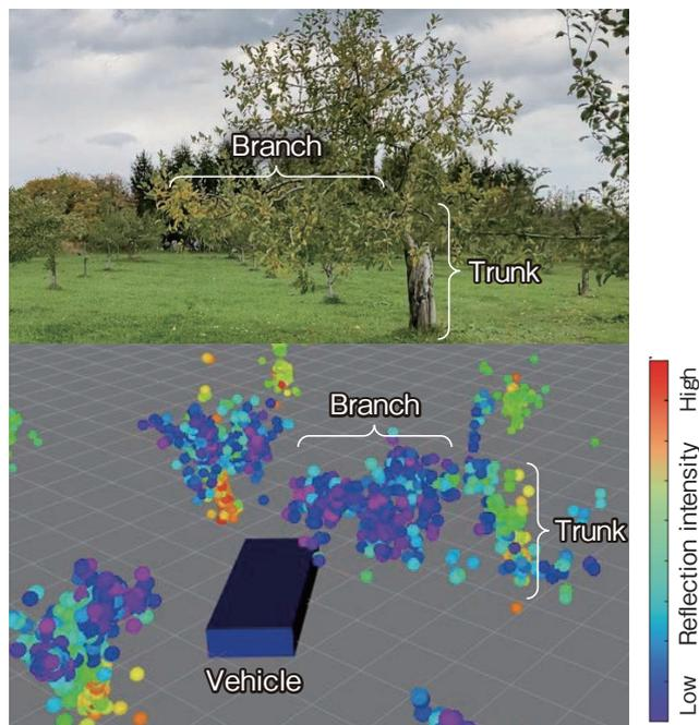
Figure 8 3D detection performance of radar.
