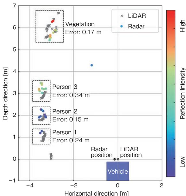
Figure 7 Comparison results of radar and LiDAR ranging performances.
