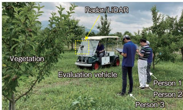
Figure 6 Evaluation view of radar and LiDAR ranging performance.
