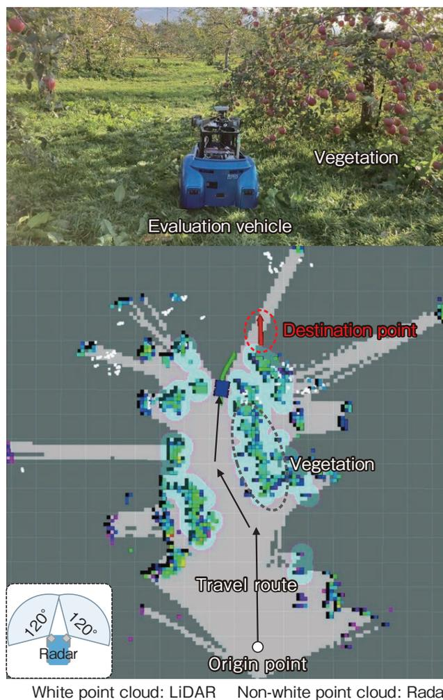
**Figure 12** Evaluation results of autonomous driving evaluation using radar.
