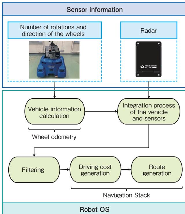
**Figure 11** Sensor configuration to an autonomous driving application.
