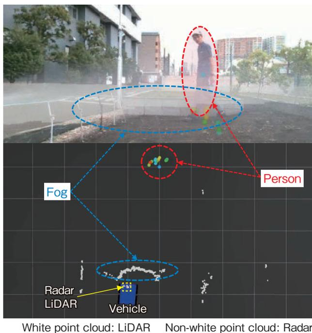
Figure 9 Comparison results of radar and LiDAR detection performance in a foggy environment.
