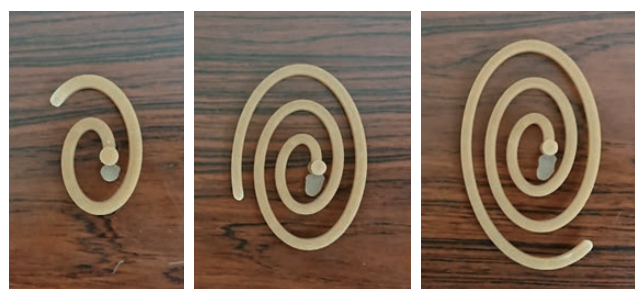
Figure 4 Examples of the spiral flow test of CELRe (from left: injection pressure 50 MPa, 100 MPa, 150 MPa).
