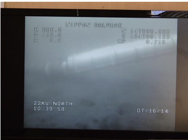
Figure 11 Submarine joint on the seabed.
