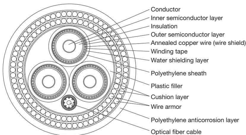
Figure 4 Structure of the 22 kV riser cable.
