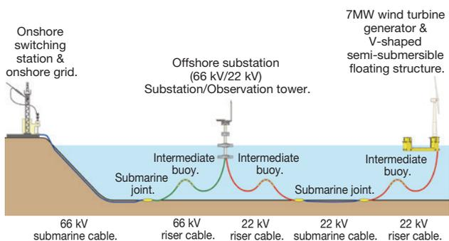
Figure 2 Transmission and substation system.
