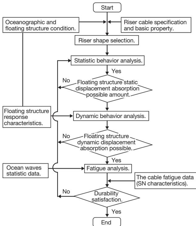
Figure 3 Designing flow of the riser cable system.
