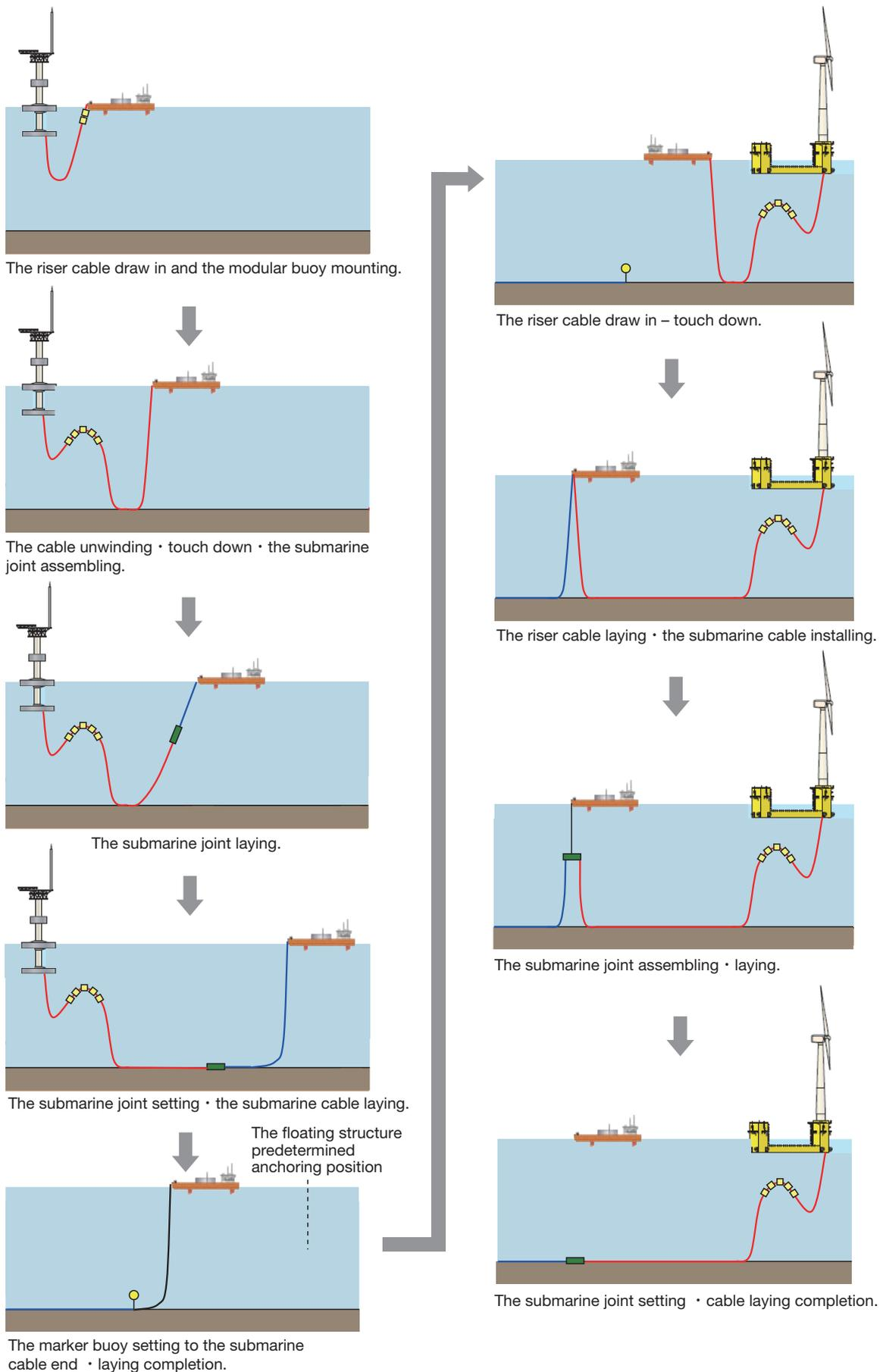
Figure 6 Cable laying procedure of the 22 kV riser cable and the submarine cable.
