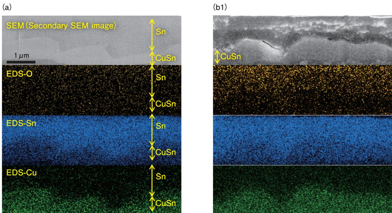
Figure 6 A SEM image of the FIB cross section of the flat test pieces and their EDS mapping images.
