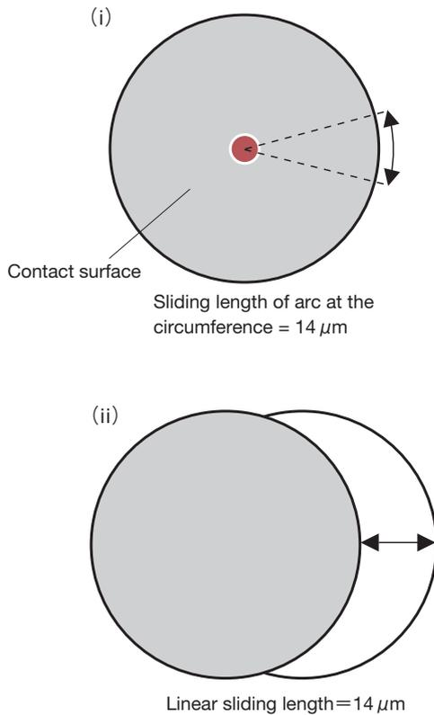
**Figure 9** Schematic sketch of the sliding length on the contact surface.
