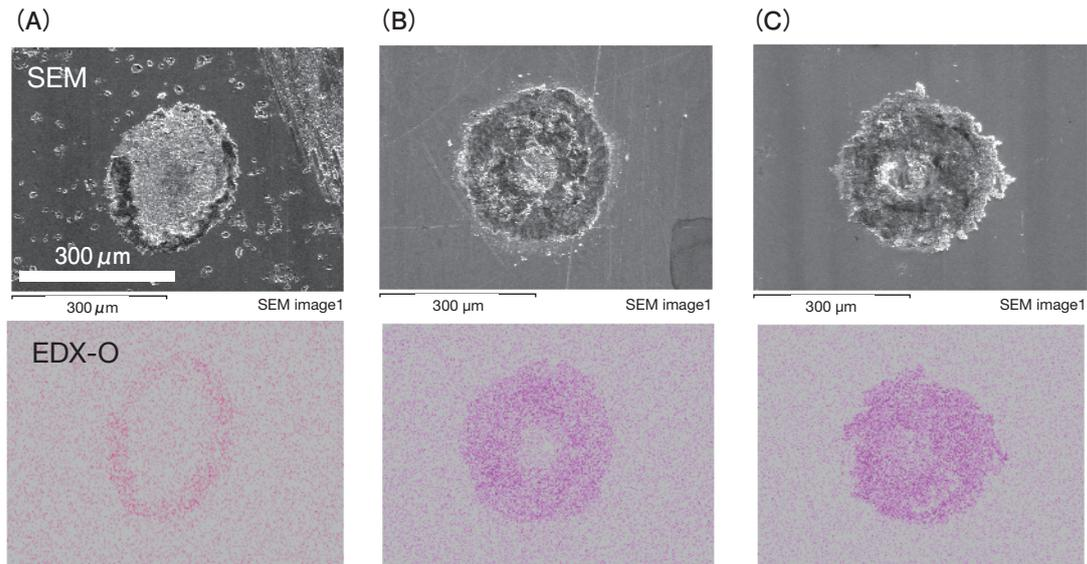
**Figure 7 SEM images of the surface of fretting trace on the flat test pieces and their EDS mapping images.**
