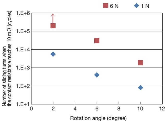
**Figure 8 Influence of the rotation angle on the number of sliding turns when the contact resistance reaches 10 mΩ.**
