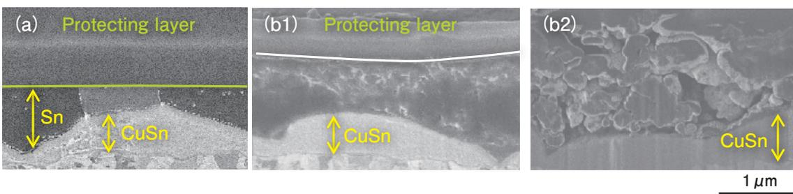
Figure 5 SIM images of the FIB cross section of the flat test pieces. (a) Before rotational sliding. (b1) and (b2) Fretting trace after rotational sliding. (Rotated under condition of 1 N, 6 degree and 100 turns.)
