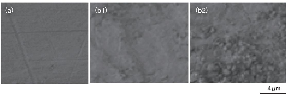
Figure 4 SIM images of the surface of the flat test pieces. (a) Before rotational sliding. (b1) and (b2) Fretting trace after rotational sliding. (Rotated under condition of 1 N, 6 degree and 100 turns.)
