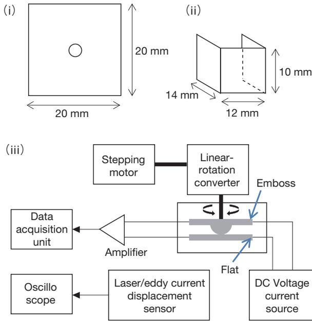
**Figure 1** (i) Embossed test piece, (ii) Flat test piece, (iii) Schematic diagram of the rotational fretting corrosion tester.
