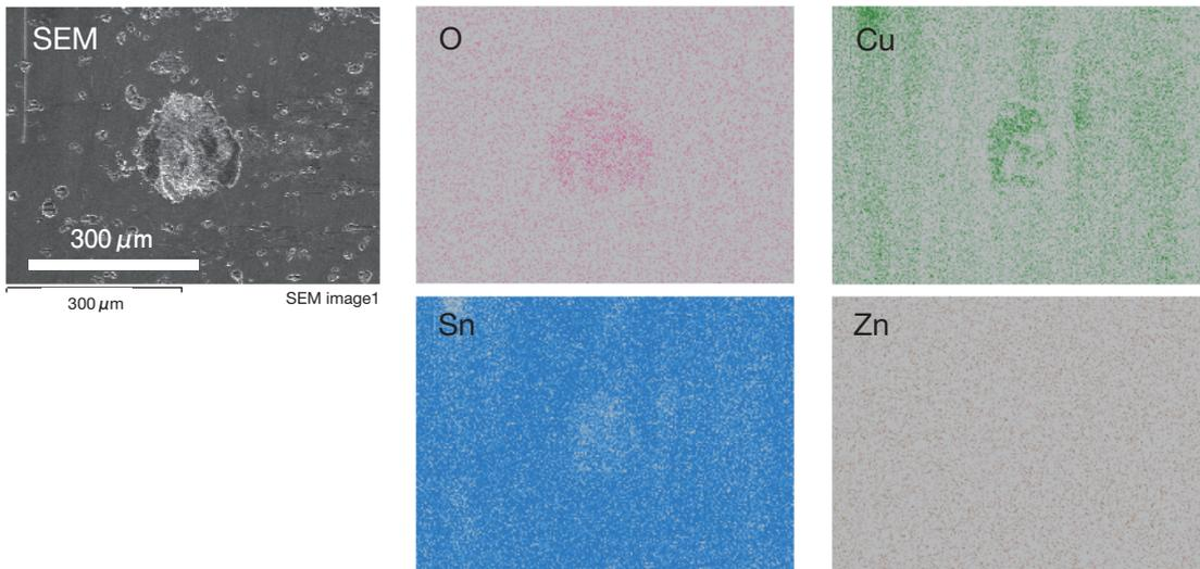
Figure 3 A SEM image of the surface of the flat test pieces and their EDS mapping images. (Rotated under condition of 1 N, 6 degree and 100 turns.)
