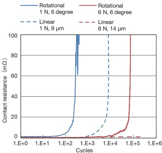
**Figure 10** Relation of the contact resistance profile against the number of rotational slidings and linear slidings. (Under condition of 1 N and 6 N.)
