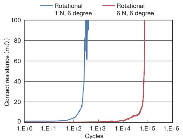
**Figure 2** Relation of the contact resistance profile against the number of rotational slidings.
