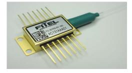
Pump source lasers for the Raman amplifier
