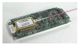
High-output, narrow-width full-band tunable laser module (ITLA)
