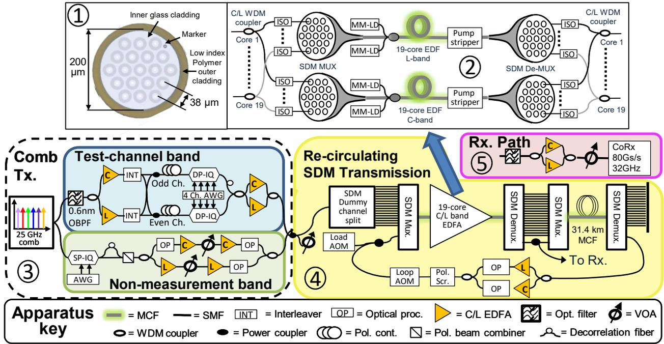
Fig.2: A schematic diagram of the 19-core EDFA and transmission system.
