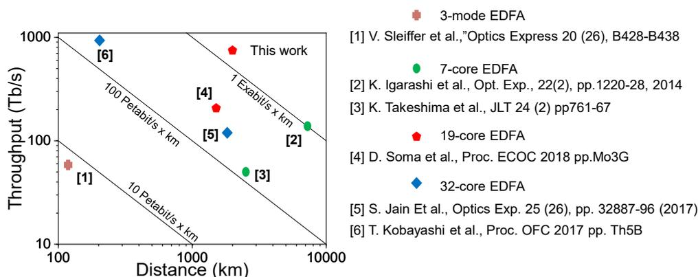
Fig.1: Comparison between our 4-core, 3-mode optical fiber and other optical fibers
